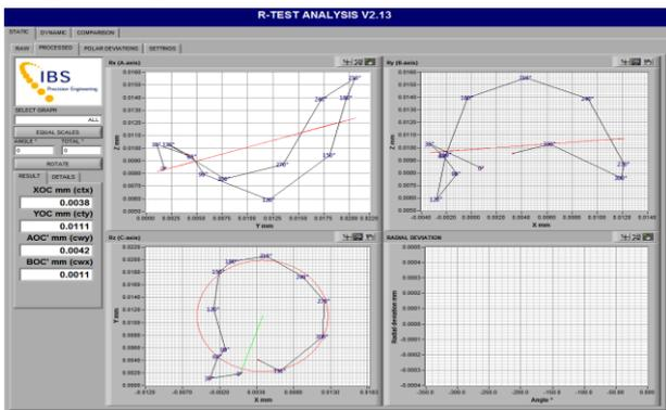
**Figure 6. Graphic representation of static measurements results**
