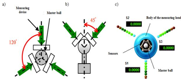
**Figure 4. MT-Probe measuring head of R-Test system [13]: a) top view, b) end view, c) bottom view**
