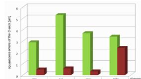
Figure 11. Changes of the squareness error of AOC axis relative to A axis and BOC relative to B axis in the function of feed motion speed  $v_f$
