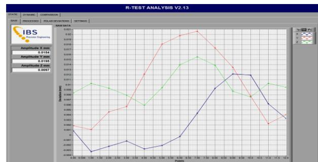
**Figure 5. Displacement of the master ball centre point making a discrete rotary motion relative to C axis in respect to the measuring head sensors during the static measurement**
