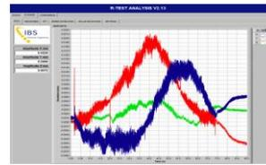
**Figure 7. The displacement of the centre point of the master ball which is in constant C rotary motion relatively to Z axis**
