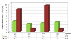
Figure 10. Changes of the kinematic centre offset error of the C rotary axis in the direction of axis X→XOC and Y→YOC
