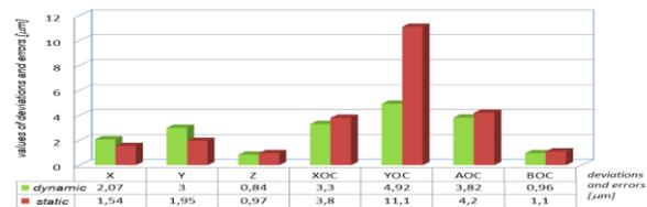
Figure 12. Comparative summary of analysed results of static measurements and mean value of errors and deviations (amplitudes) from dynamic measurements
