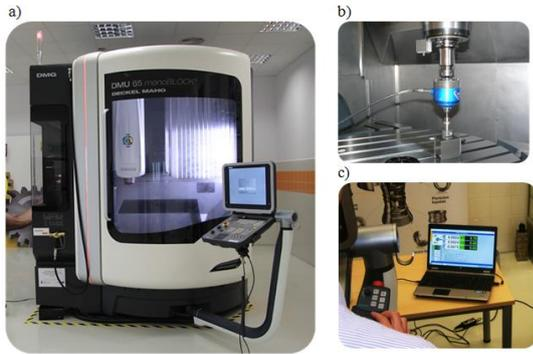
**Figure 1.** Test object: a) vertical 5-axis machining centre DMU 65 MonoBlock by DMG company, b) R-Test measuring system by IBS Precision Engineering, mounted on the machine tool, c) computer operating MTS-003 software.
