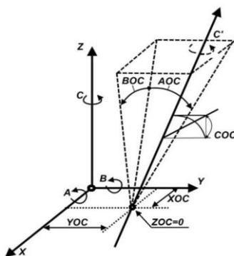
**Figure 2.** Kinematic centre offset errors of the C rotary axis
