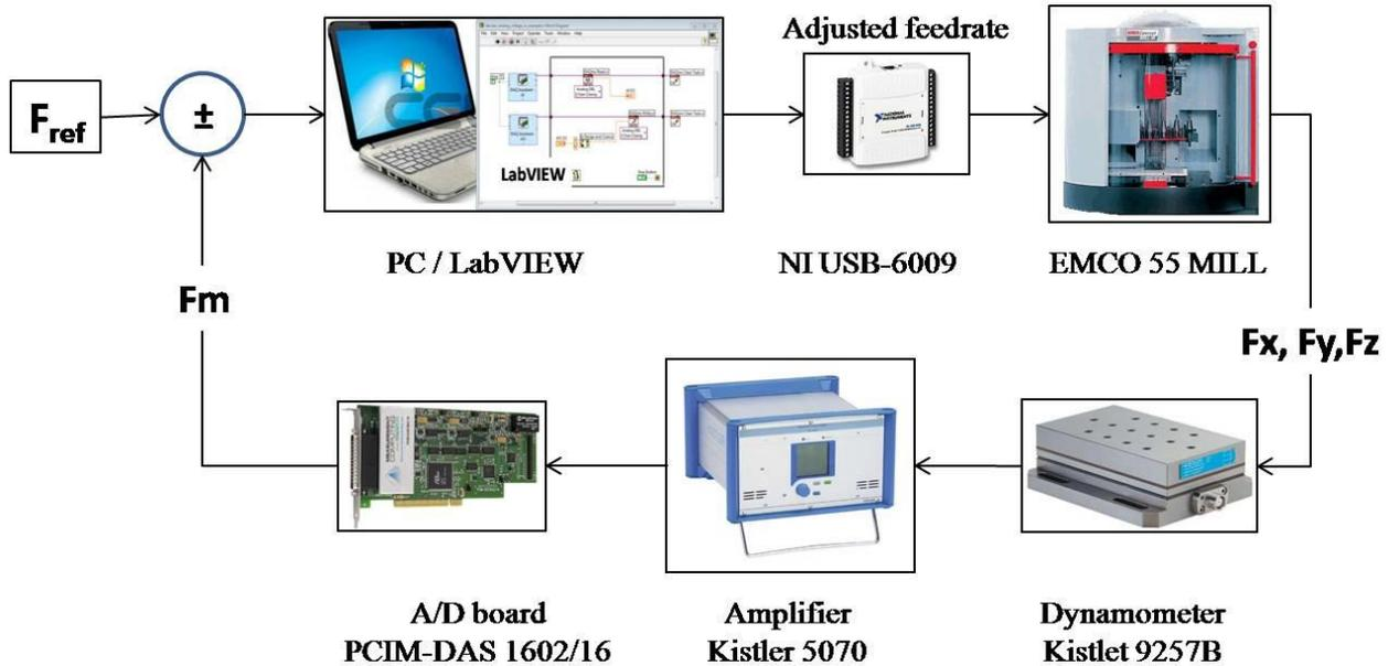
Figure 3. Hardware architecture
