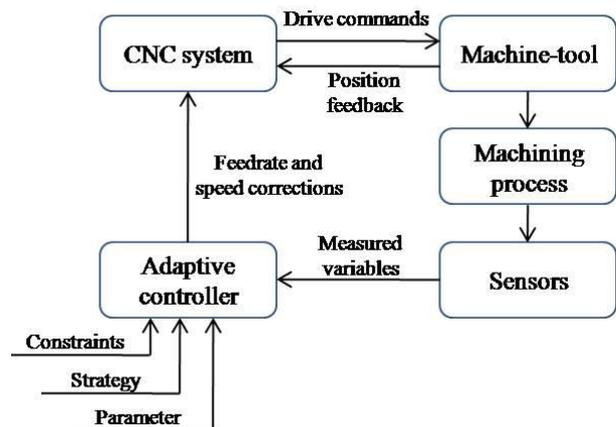
Figure 1. Adaptive control system for CNC machine-tool
