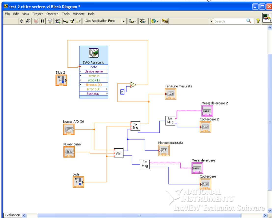
Figure 7 LabVIEW Virtual Instrument for gathering data from Kistler dynamometer and delivering corrections to machine-tool Overwrite knob
