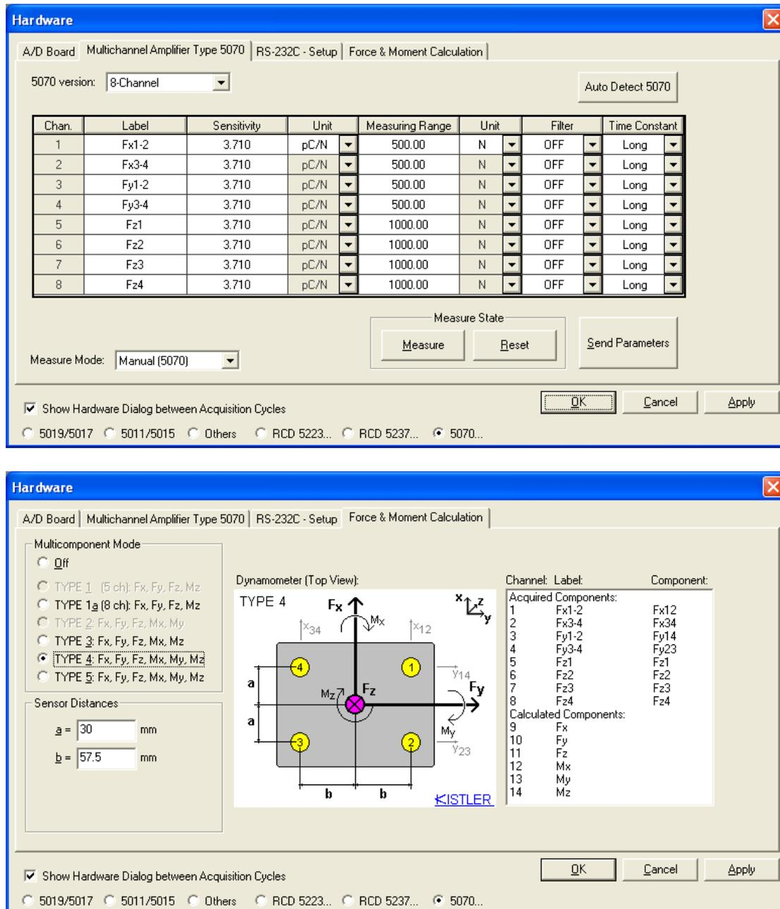
Figure 5. Dynamometer and Amplifier configuration
