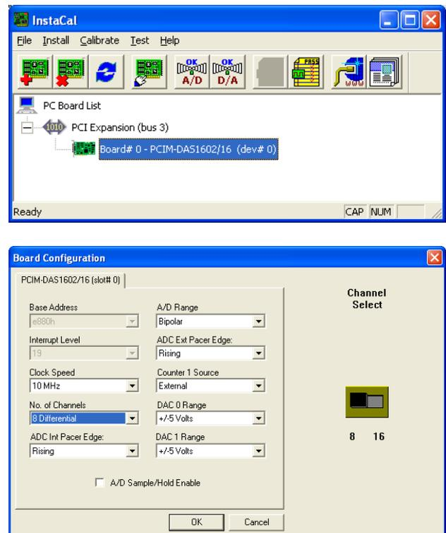
Figure 4. A/D board configuration
