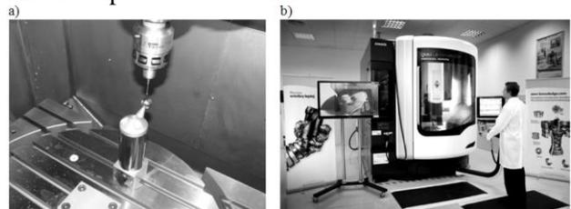
**Figure 7. Installation of DMG 3D quickSET calibration system**
