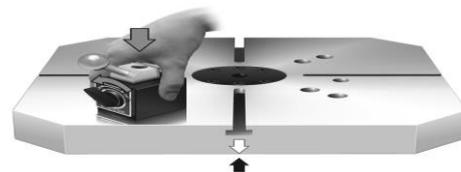
**Figure 4. Mounting the master ball on the machine tool table [16]**
