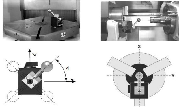
**Figure 3. AxiSet™ Check-Up by Renishaw during C-axis calibration:** a) on a mill, b) on a lathe, c) mounting the ball on a mill, d) mounting the ball on a lathe [16]
