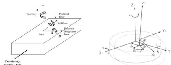
**Figure 1. Linear and rotational axis errors:**
