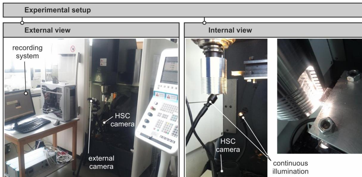
**Figure 3. Experimental setup**
