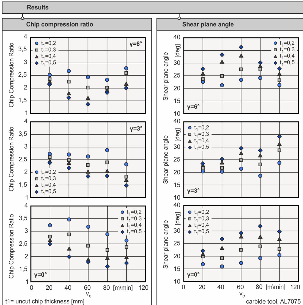
Figure 5. Results of chip formation characteristics
