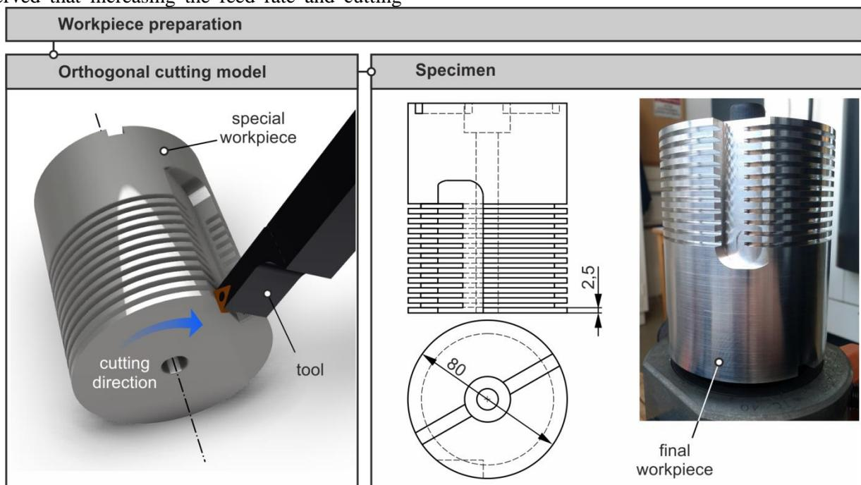
Figure 2. Special workpiece (AL7075) preparation
