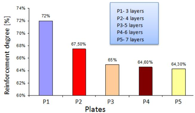
Figure 4 The influence of the number of layers of reinforcement degree
