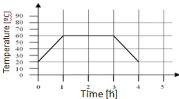
Figure 3. Temperature/time composite polymerization diagram
