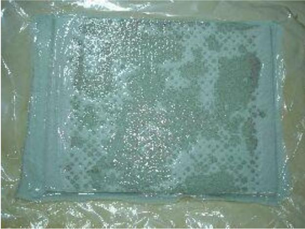
Figure 2. The vacuum applied to the mould determine the elimination of resin excess
