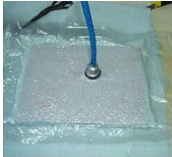
Figure 1. The vacuum applied to the mould After vacuum applied all the excess of the resin penetrated the perforated folia and absorbed in textile material. The applied pressure on wet composite material is constant. The air bubble from composite is eliminating and the excess of resin (Figure 2).
