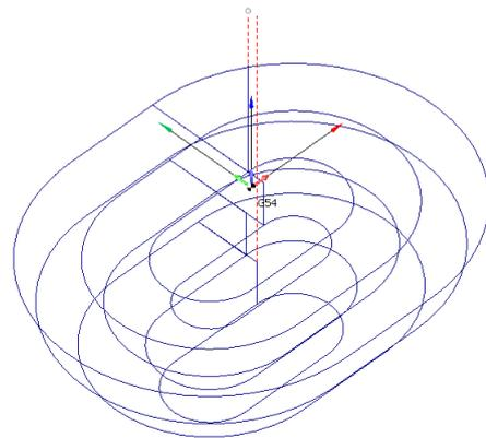
Figure 2. Toolpaths for operation A (roughing)
