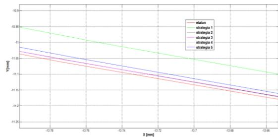
Figure 13. Graphical display of the accuracy of the machine parte (curves at 45°, detail)
