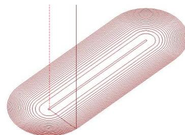
Figure 3. Toolpaths for operation C (supplementary finishing)
