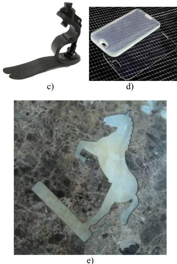
Fig.1. Parts made by AWJ cutting technology; a) Aluminum; b) Cooper; c) Composites material reinforced with fibre; d) Glass; e) Marble pattern, made at TUCN, (Omax)
