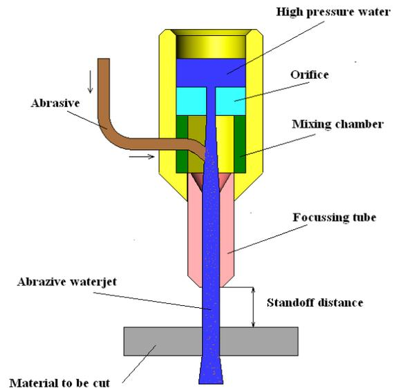
Fig.2. Working principle of WJC process
