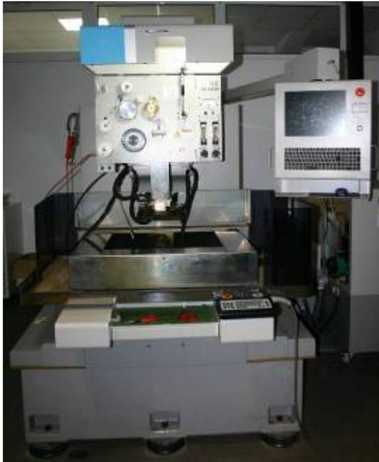
Fig.3. EDM Wire Cutting Equipment, SP-640P, TUCN
