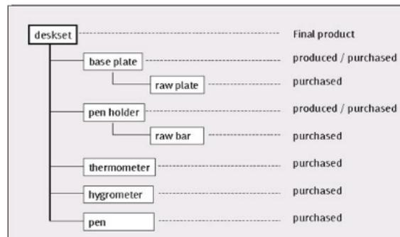
Fig.5. Parts list structure. Source: (Festo Spol. SR., 2012)
