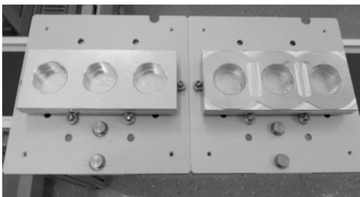
Fig.8. Default baseplate shape (on the left) and manufactured penholder after having modified its default shape using the CAD/CAM software of iCIM 3000. Source: IPSAM archives.
