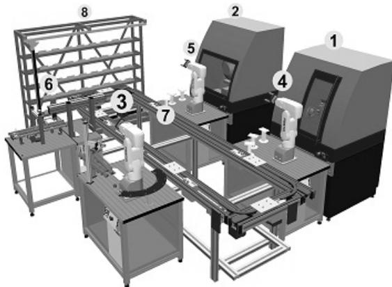
Fig.4. 3D layout configuration of the iCIM 3000 at the IPSAM. Source: Self-elaboration.
