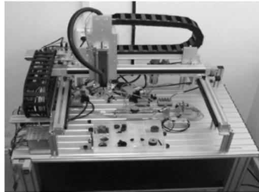
Fig.2. Cartesian robot station for the assembly-disassembly. Source: (Danišová et al. 2012)
