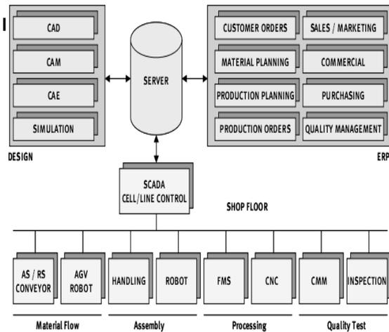
Fig.3. General framework for the iCIM 3000 functioning. Source: (Festo Spol. SR., 2012)
