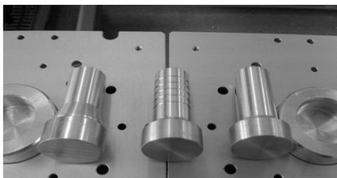
Fig.7. Default penholder shapes and new manufactured penholder after having modified its shape using the CAD/CAM software of iCIM 3000 (the first one on the left). Source: IPSAM archives.
