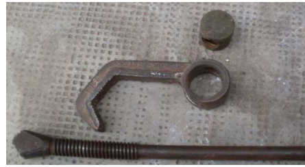
Fig.10. Screw trimowrench, subject of case study (Pescaru & Oancea, 2012)
