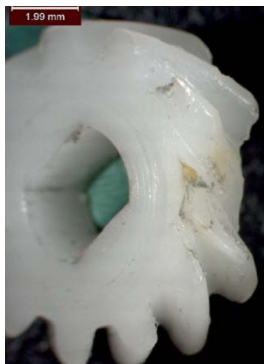
Fig.2. Damaged gear (Manolescu et al., 2011)
