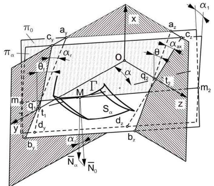
Fig.4. The characteristic triangular planes of generating cutting processes
