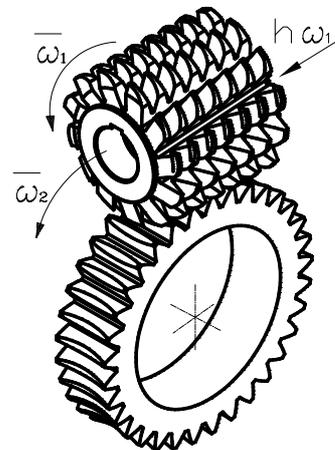
Fig.1. The position and relative movements within virtual gear manufacturing
