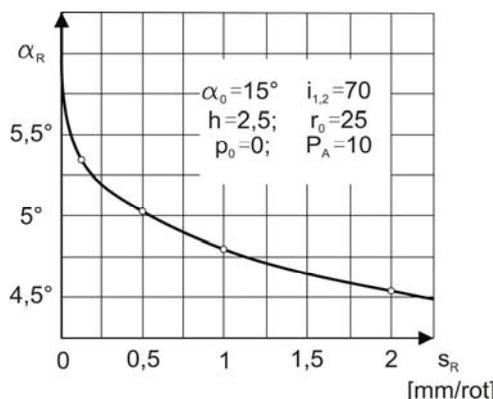
Fig.6. The variation of the functional lateral clearance angle
