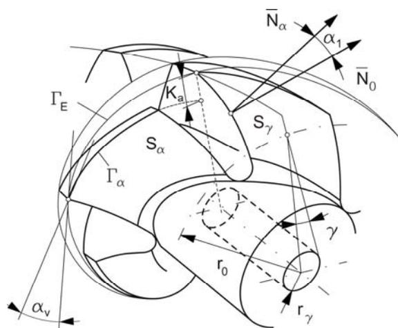
Fig.2. The constructive geometry of worm-hob
