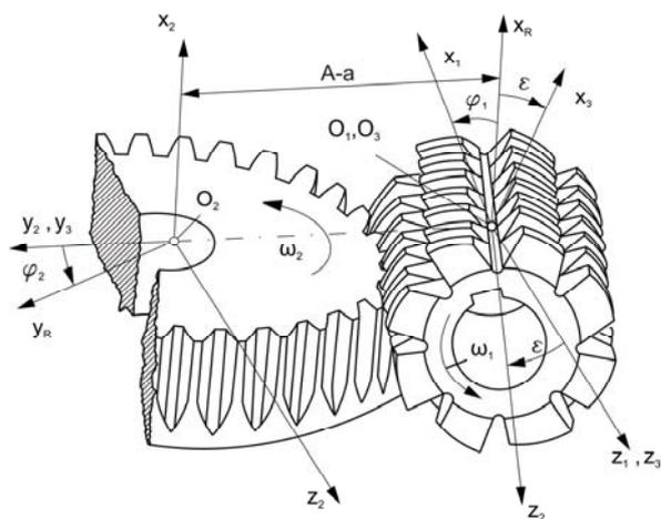
Fig.5. Relative position and movement between worm-hob gear in the cutting processes
