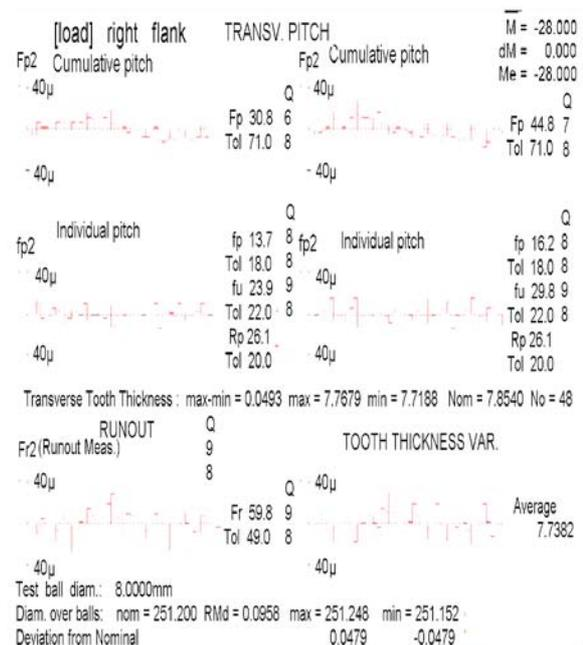
Fig.9. Run out and pitch evaluation chart
