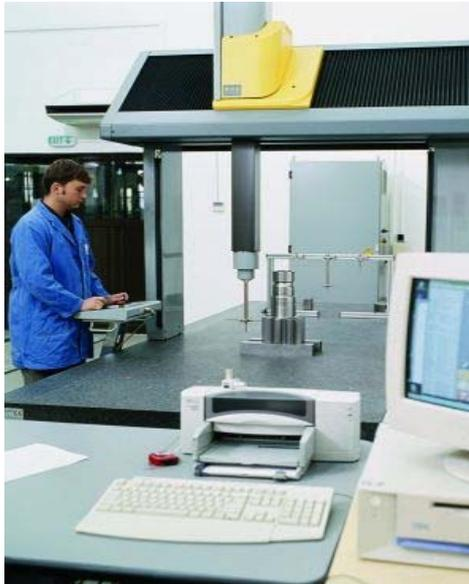
Fig.7. Measurement of worm wheels for cylindrical worms on Brown&Sharpe ghibli-trax
