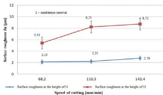
Fig.6. The influence of abrasive water jet cutting speed on surface roughness parameter  $R_a$
