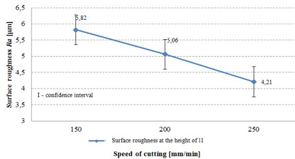
Fig.8. Influence of laser beam cutting speed on the surface roughness parameter  $Ra$
