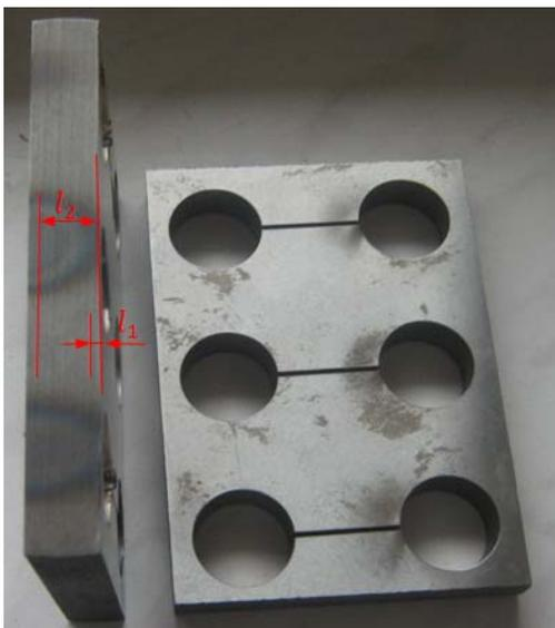
Fig.1. Holes diameter measurement locations; measured from the side of the concentrated energy beam incidence
