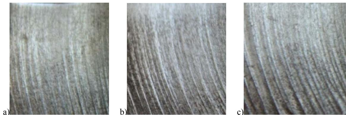
Fig.7. Photographs of holes surfaces after abrasive water jet cutting for cutting speeds of: a) 68,2 mm/min; b) 110,3 mm/min; c) 143,4 mm/min
