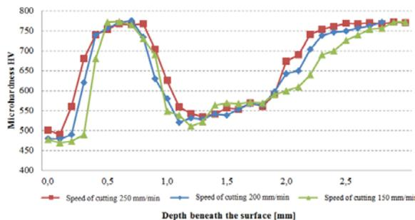
Fig.11. HV microhardness of the surface layer of NC6 steel processed with a laser beam
