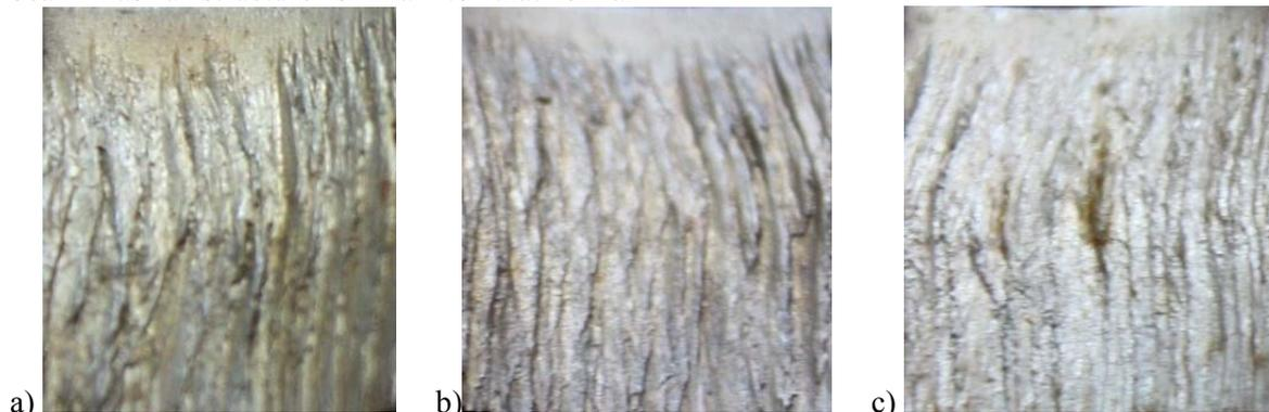
Fig.9. Photographs of holes surfaces after laser beam cutting for cutting speeds of: a) 150 mm/min; b) 200 mm/min; c) 250 mm/min
