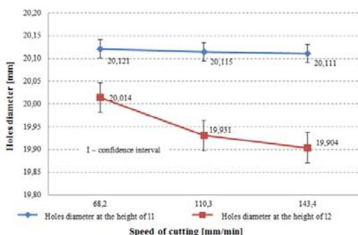
Fig.2. The influence of abrasive water jet cutting speed on the diameter  $D$  of the executed holes
