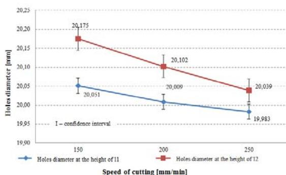
Fig.3. The influence of laser beam cutting speed on the diameter  $D$  of the executed holes
