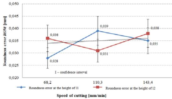
Fig.4. The influence of abrasive water jet cutting speed on the average values of roundness deviations  $RON_t$
