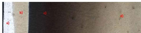
Fig.10. Arrangement of heat affected zones of NC6 steel cut with a laser beam: a) melted zone, b) secondarily hardened zone, c) tempered zone, d) core
