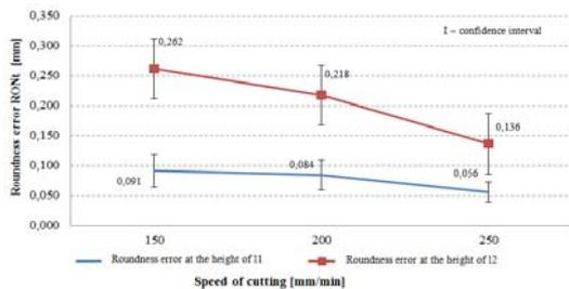
Fig.5. The influence of laser beam cutting speed on the average values of roundness deviations  $RON_t$
