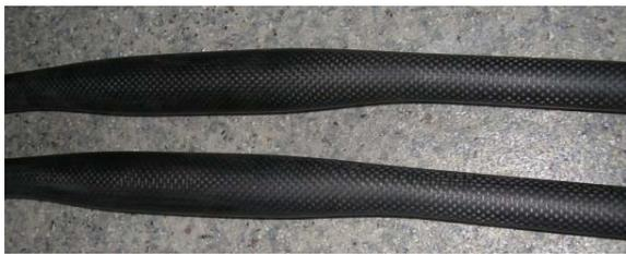
Fig.7. The handlebars form carbon fibre
