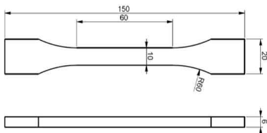
Fig.8. The dimensions of specimens [STAS SR EN ISO 527-4]
