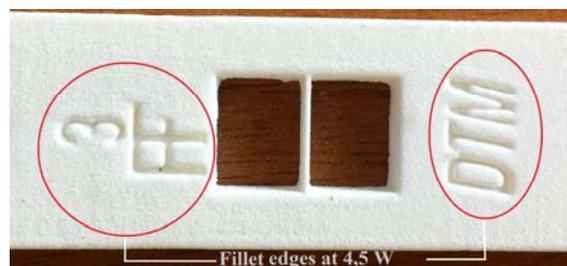
Fig.6. Part from PA 2200 powder produced at 4.5 W
