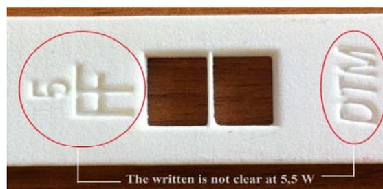
Fig.7. Part from PA 2200 powder produced at 5.5 W
