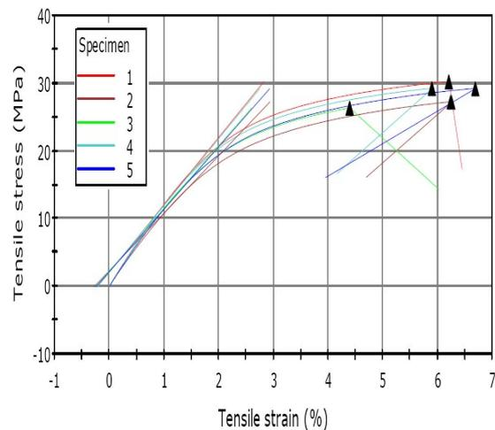
Fig.9. Variation of tensile stress with tensile strain for specimens made at 3,5 W laser power
