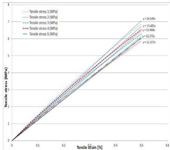
Fig. 12. Determination of E-modulus for specimens made at 3,5 W laser power
