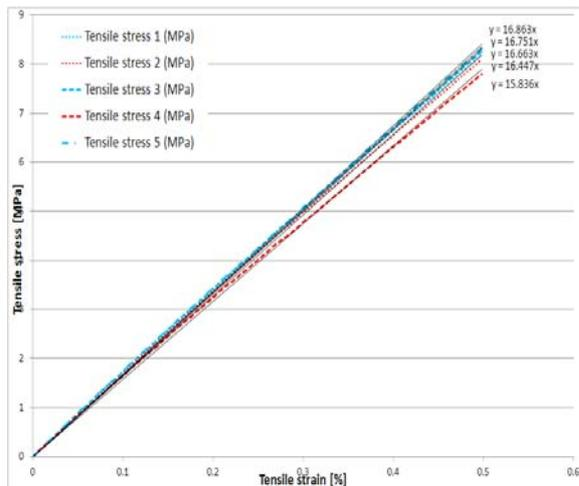
Fig.13. Determination of E-modulus for specimens made at 4 W laser power
