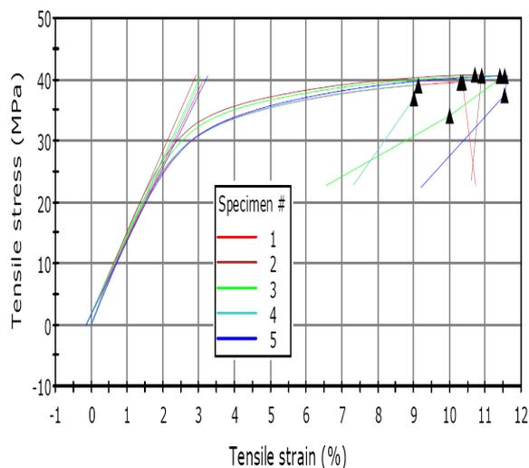
Fig. 11. Variation of tensile stress with tensile strain for specimens made at 4,5 W laser power
