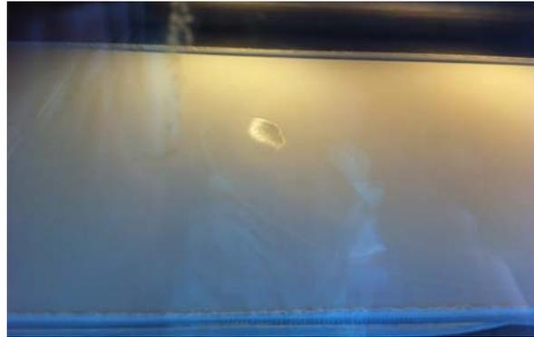
Fig.1. PA 2200 powder at 183°C temperature
