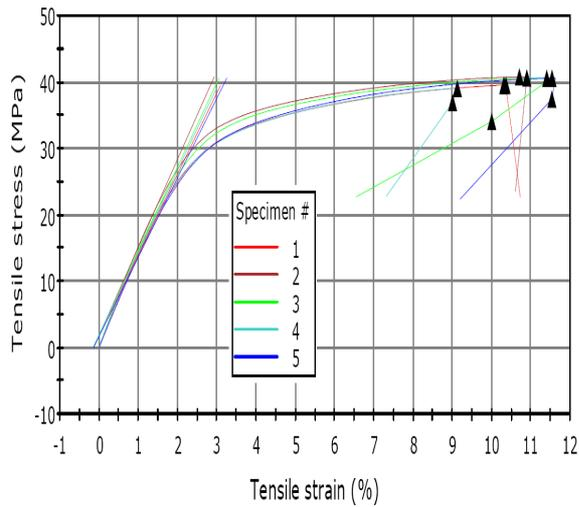
Fig. 10. Variation of tensile stress with tensile strain for specimens made at 4 W laser power
