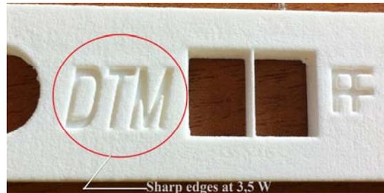
Fig.5. Part from PA 2200 powder produced at 3.5 W
