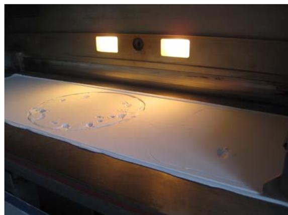
Fig.2. Picture inside the machine Sinterstation 2000 after processing the first test pieces from PA 2200 powder
