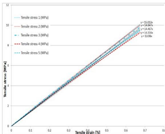
Fig.14. Determination of E-modulus for specimens made at 4,5 W laser power
