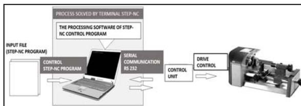
Fig.11. Process of data transmission to the control unit Lathe - Emco Unimat PC
