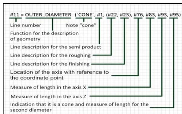
Fig.9. Structure description of one program line Data decoded from the input file STEP-NC with this proposed procedure, are then allocated to a geometric object and transform to the necessary
