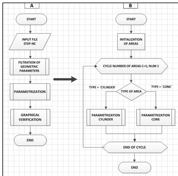
Fig.10. A: Flowchart of decoding STEP-NC data
