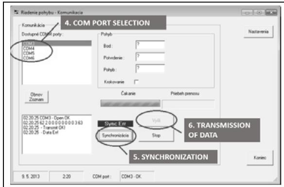
Fig.13. Procedure for realization of communication
