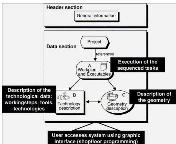
Fig.4. Structure of the STEP-NC data model (Xu, X.W. 2006)
