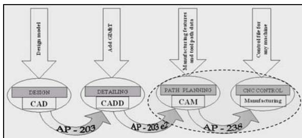
Fig.2. Data flow with the using of STEP-NC
