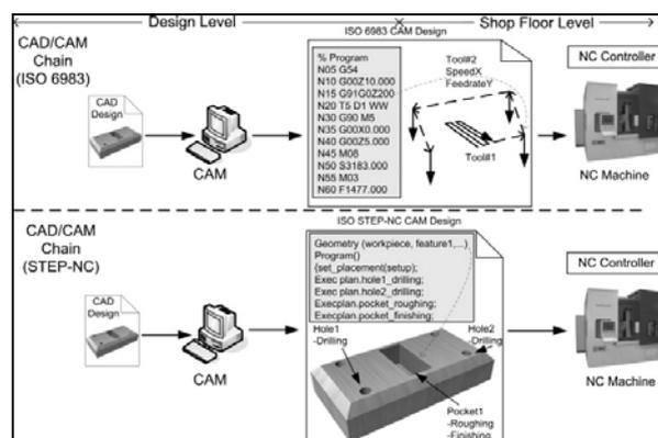
Fig.3. Comparison between programming with G&M codes and STEP-NC (Campos J.G. & Miguez,L.R., 2011)
