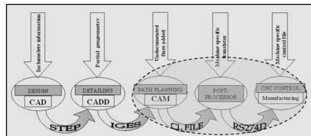
Fig.1. Current NC Programming Interface
