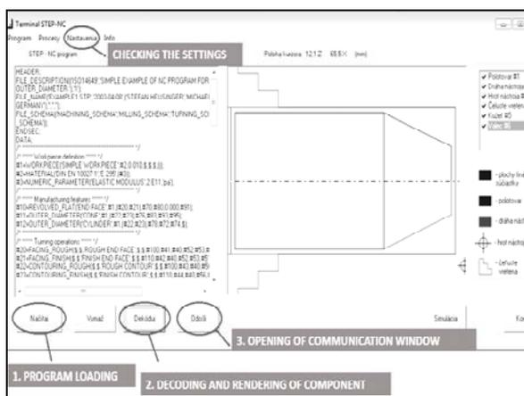
Fig.12. Procedure for processing of STEP-NC
