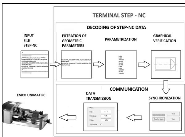
Fig.7. Working principle of software - TERMINAL STEP-NC
