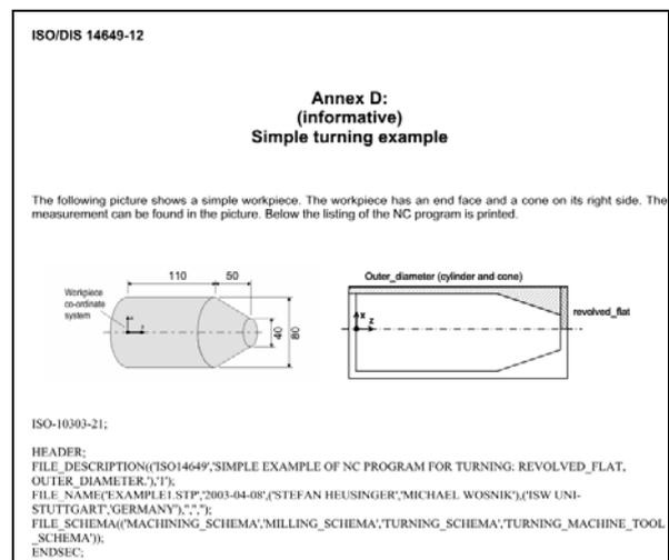
Fig.8. List of control program for turning example from Standard - ISO 14649-12
