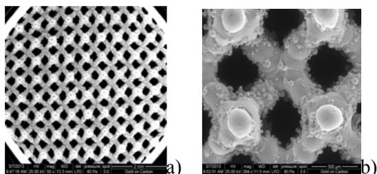
Fig.4. Disc with cell –size 0.6 mm, before infiltration; a) 50x, b) 284x magnification
