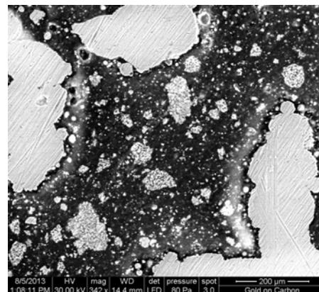
Fig.9. Disc with cell –size 1 mm, after infiltration with paste P2; 350x magnify
