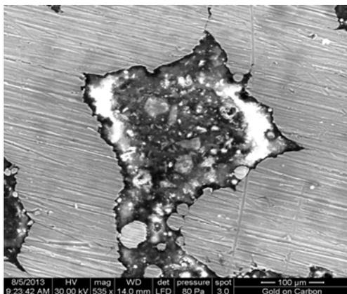
Fig.7. Disc with cell –size 0.6 mm, after infiltration with paste P1; 535x magnify
