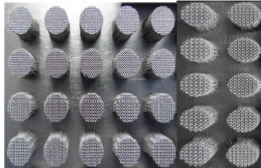
Fig.1. Discs with 5 different porosities, manufactured on the MCP Realizer II SLM 250
