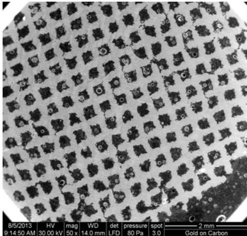
Fig.6. Disc with cell –size 0.6 mm, after infiltration with paste P1; 50x magnify
