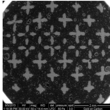
Fig.8. Disc with cell –size 1 mm, after infiltration with paste P2; 50x magnify
