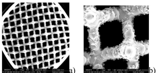
Fig.5. Disc with cell–size 1mm, before infiltration; a) 51x, b) 294x magnification
