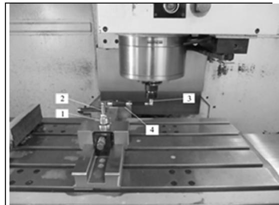
Fig.1. Measuring device Ballbar QC20 – 1. Magnetic center holder, 2. Magnetic centre cup attached to rack, 3. Magnetic centre cup clamped in collet, 4. Measuring device
