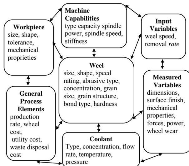
Fig.1. The process elements for surface grinding (Shaw, 1996)
