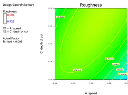
Fig.14. The variation of roughness relative to  $v$ ,  $a_p$ ,  $f = 0.008$  mm/rev
