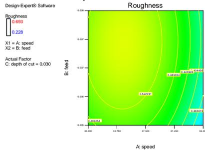
Fig.6. The variation of roughness relative to  $v, f$
