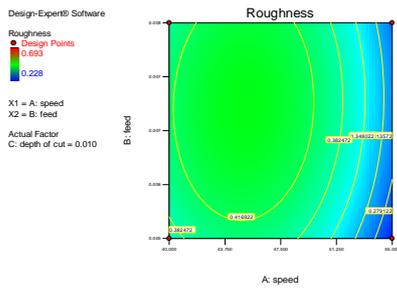
Fig.5. The variation of roughness relative to  $v, f$
