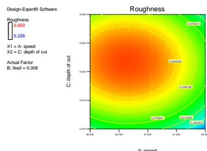
Fig.8. The variation of roughness relative to  $v, a_p, f = 0.008 \text{ mm/rev}$
