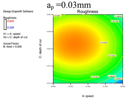
Fig.7. The variation of roughness relative to  $v, a_p, f = 0.005 \text{ mm/rev}$
