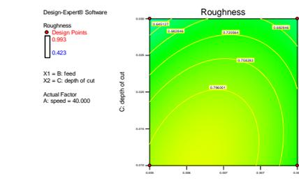
Fig.15. The variation of roughness relative to  $f$ ,  $a_p$
