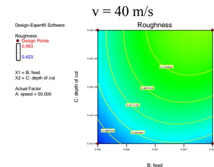
Fig.16. The variation of roughness relative to  $f$ ,  $a_p$ ,  $v = 55$  m/s
