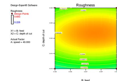
Fig.9. The variation of roughness relative to  $f, a_p$
