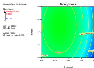
Fig.11. The variation of roughness relative to  $v, f$
