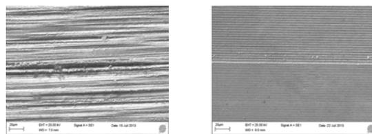
a) Surface before processing b) machined surface  $v = 40$  m/s,  $f = 0.008$  mm/rev,  $a_p = 0.03$  mm
