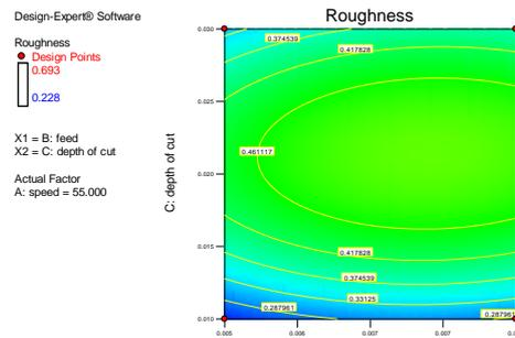
Fig.10. The variation of roughness relative to  $f, a_p$
