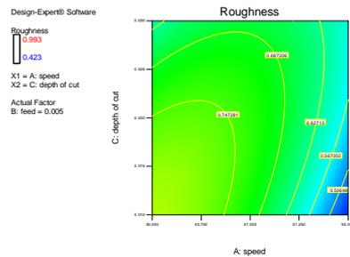
Fig.13. The variation of roughness relative to  $v$ ,  $a_p$ ,  $f = 0.005$  mm/rev
