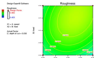
Fig.12. The variation of roughness relative to  $v$ ,  $f$ ,  $a_p=0.03$ mm
