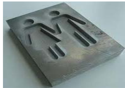
Fig.1. Part made by AWJ milling (Omax)
