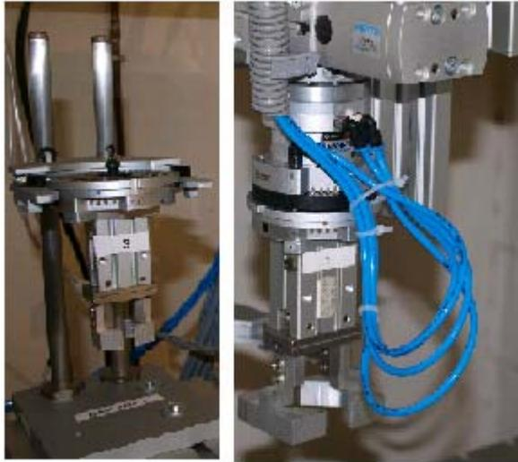
Fig.13. Utilization of reed sensor in the intelligent assembly cell
