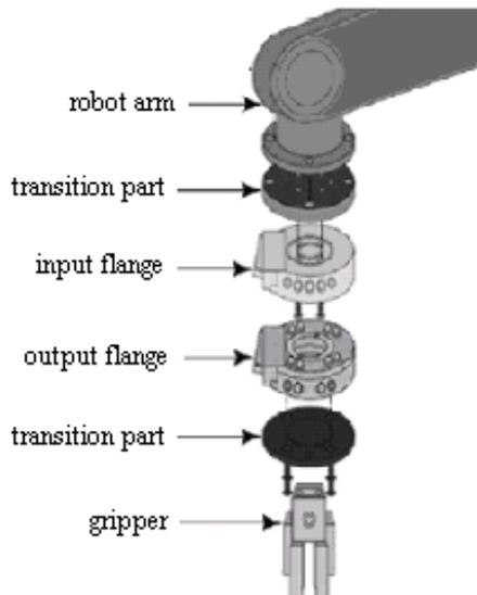
Fig.8. The bind of exchange gripper
