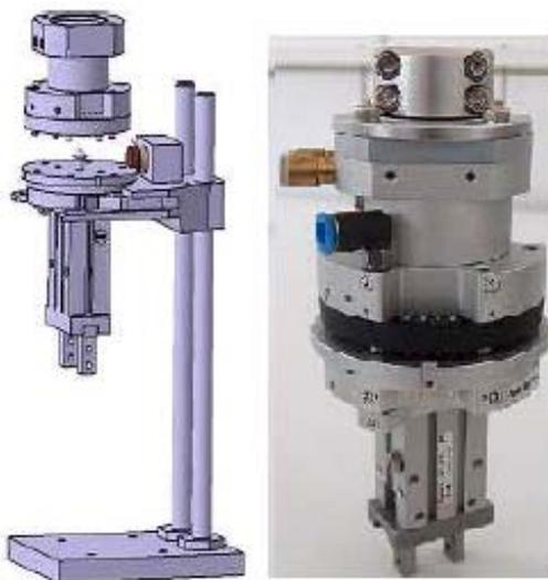
Fig.9. The scheme and real example of exchange gripper
