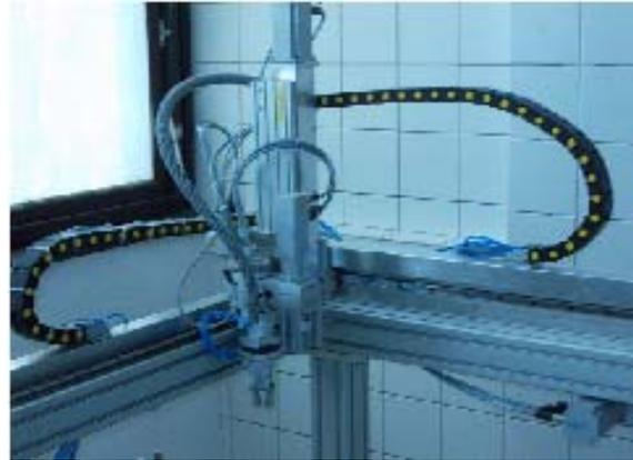
Fig.6. External robot with Cartesian coordinate system in the assembly workspace
