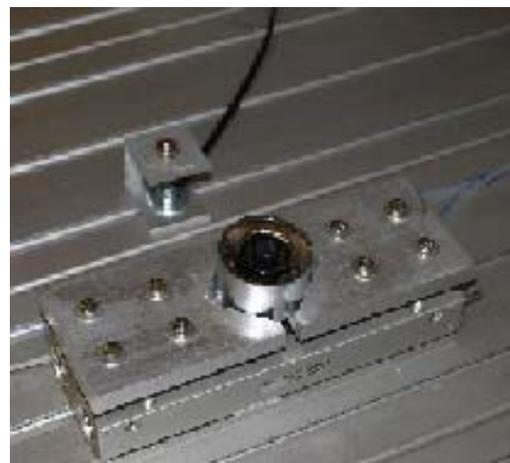
Fig.11. Utilization of optical sensor with suppressed background in the intelligent assembly cell
