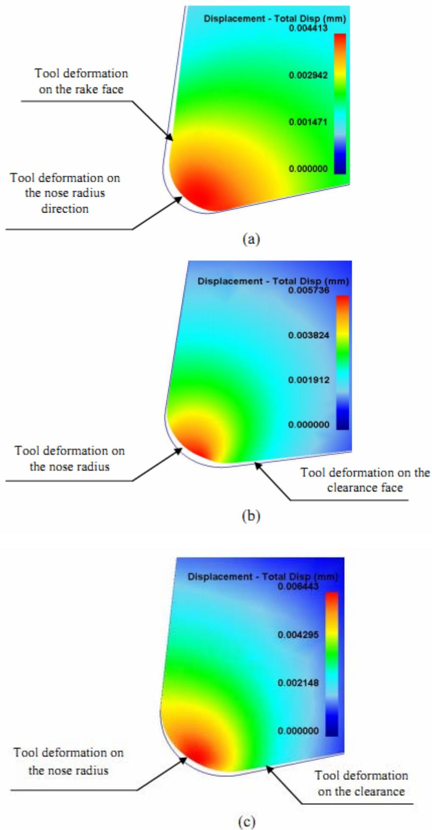
Fig.1. Thermal deformation of the cutting tool: (a) for  $r_\beta=0.4\text{mm}$ ; (b) for  $r_\beta=0.8\text{mm}$ ; (c) for  $r_\beta=1.2\text{mm}$ .
