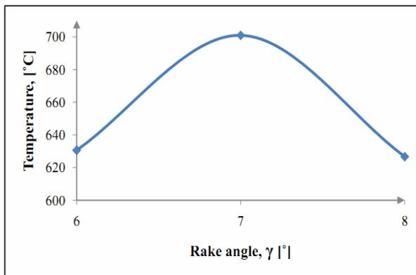
Fig.3 Variation of the temperature with rake angle.
