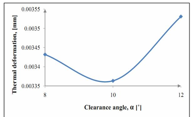
Fig.7. Variation of the thermal deformation with clearance angle.
