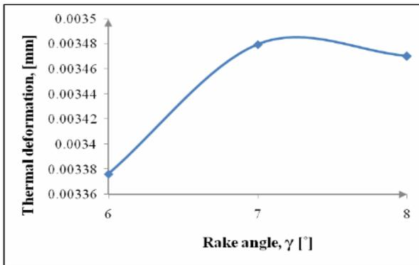
Fig.4. Variation of the thermal deformation with rake angle.
