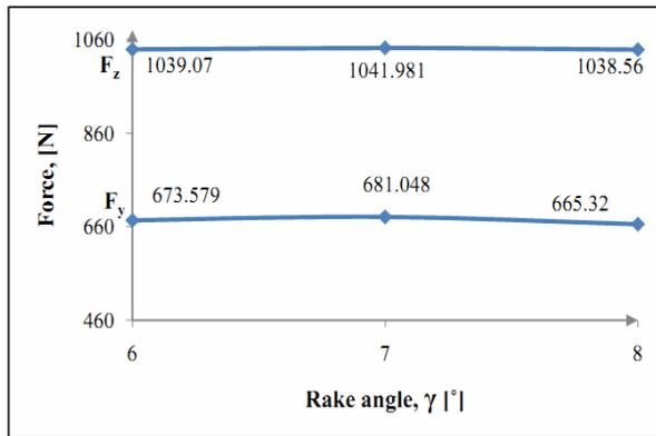
Fig.2. Variation of the cutting forces with rake angle.
