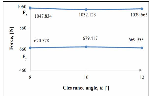
Fig.5. Variation of the cutting forces with clearance angle.
