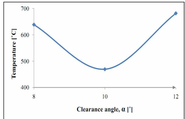
Fig.6. Variation of the temperature with clearance angle.
