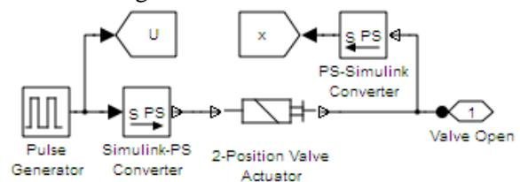
Figure 3. Functional subsystem for modeling the “Electromagnetic Actuator”
