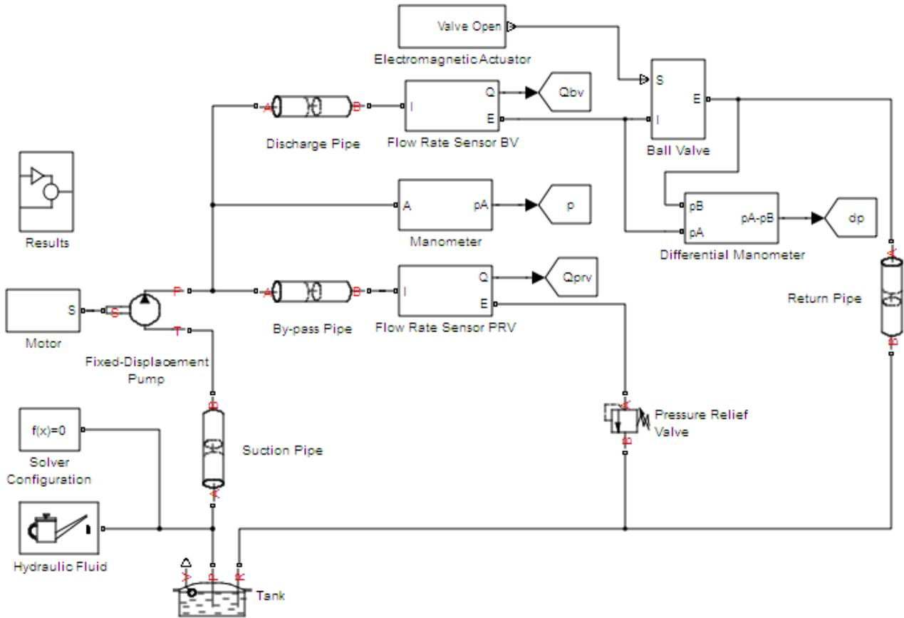
Figure 1. Functional diagram for modeling the electromagnetic ball valve with conical seat
