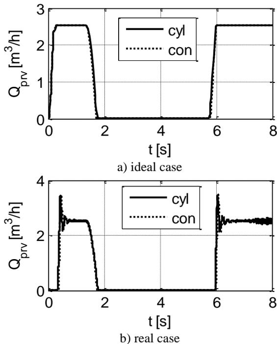
Figure 18. Comparative volumetric flow rate through the pressure relief valve
