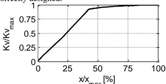
Figure 11. Dimensionless valve flow factor for ball valve with conical seat, (ideal case)
