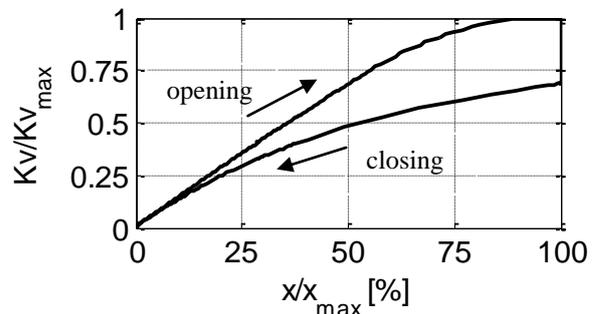
Figure 12. Dimensionless valve flow factor for ball valve with conical seat (real case)
