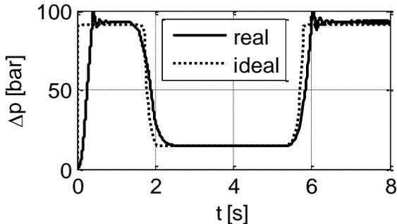
Figure 15. Pressure drop in the ball valve with conical seat
