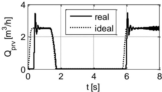
Figure 14. Volumetric flow rate through the pressure relief valve
