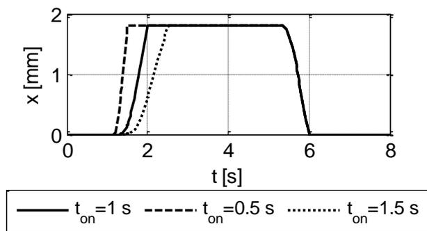
Figure 5. The influence of the switching-on time on the push-pin motion signal
