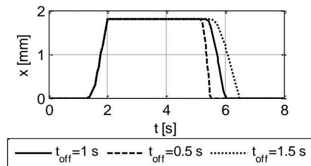
Figure 6. The influence of the switching-off time on the push-pin motion signal
