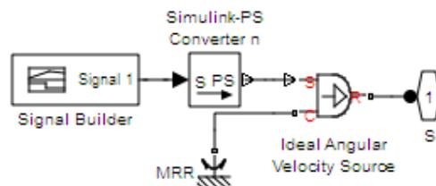
Figure 7. Functional subsystem for modeling the pump motor
