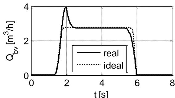
Figure 13. Volumetric flow rate through the ball valve with conical seat
