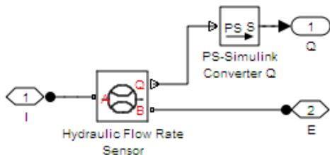
Figure 9. Functional subsystem for modeling the “Flow Rate Sensor PRV”
