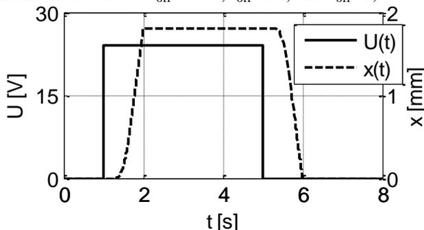
Figure 4. Input and output signals of the electromagnetic actuator
