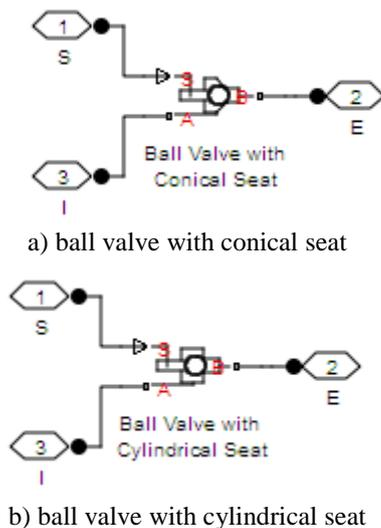
Figure 2. Functional subsystem for modeling the ball valve
