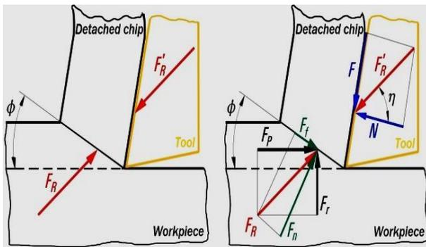
Fig.5 The forces in orthogonal cutting process
