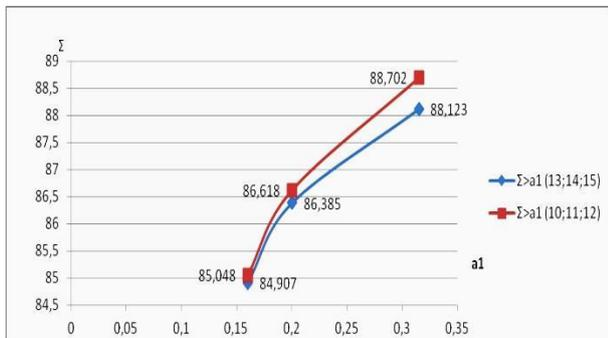
Fig.23 The influence of the attached chip's thickness  $a_{1[mm]}$  on the specific shear deformation  $\epsilon$
