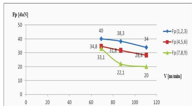
Fig.12 The influence of cutting speed  $v$  on the main cutting force (component)
