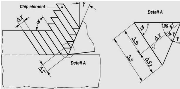
Fig.2 Merchant model of chip formation
