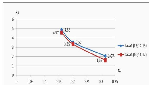
Fig.11 The influence of the attached chip's thickness  $a_1$  on chip compression
