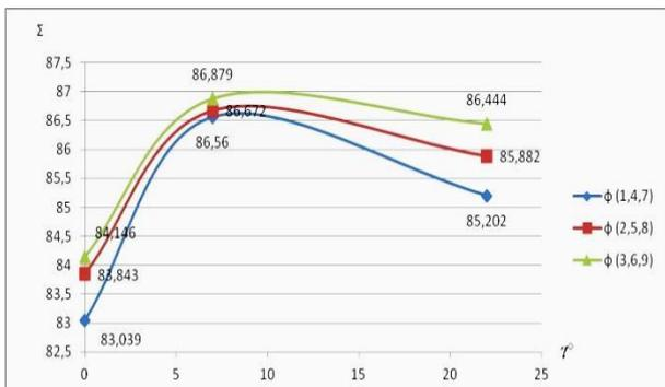
Fig.22 The influence of the rake angle  $\gamma^\circ$  on the specific shear deformation  $\epsilon$
