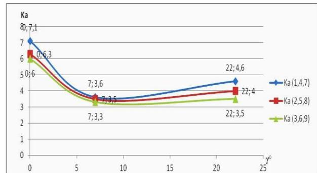
Fig.10 The influence of rake angle  $\gamma$  on chip compression
