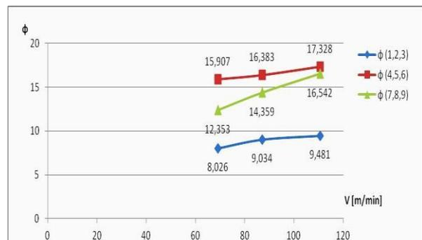
Fig.18 The influence of cutting speed  $v$  on the shear angle  $\phi$
