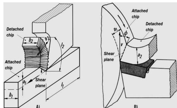
Fig.1 Orthogonal cutting:
