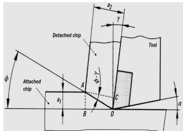
Fig.4 Geometrical necessary elements for determination of the shear angle  $\phi$
