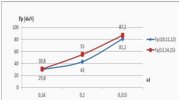
Fig.14 The influence of the attached chip's thickness  $a_1$  [mm] (feed) on the main cutting force
