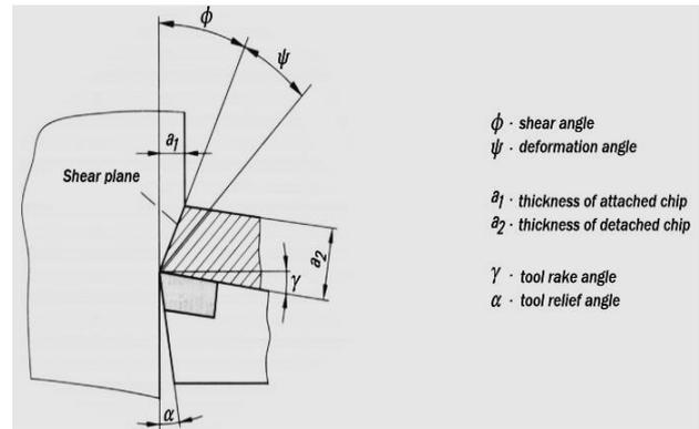
Fig.3 New orientation direction of the workpiece's crystals in the detached chip
