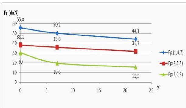
Fig.16 The influence of the rake angle  $\gamma^\circ$  on the reaction force
