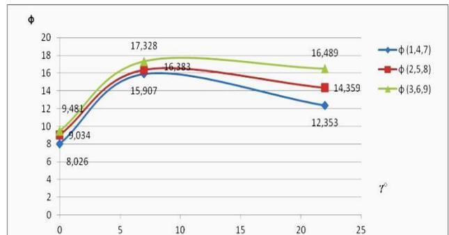
Fig.19 The influence of the rake angle  $\gamma^\circ$  on the shear angle  $\phi$
