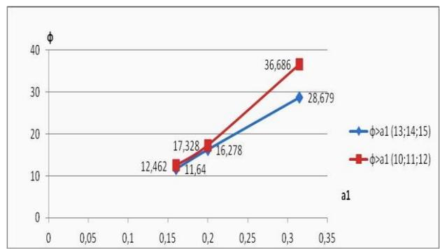
Fig.20 The influence of the attached chip's thickness  $a_1$  [mm] on the shear angle  $\phi$
