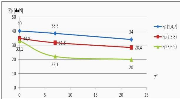
Fig.13 The influence of rake angle  $\gamma^\circ$  on the main cutting force (component)
