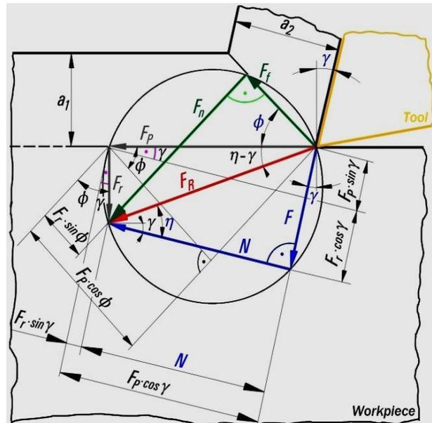
Fig.6 The diagram of orthogonal cutting forces (Merchant's circle)
