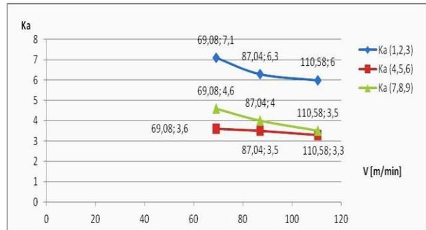
Fig. 9 The influence of cutting speed  $v$  on chip compression
