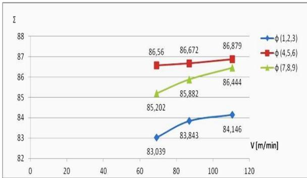
Fig.21 The influence of cutting speed  $v$  on the specific shear deformation  $\epsilon$
