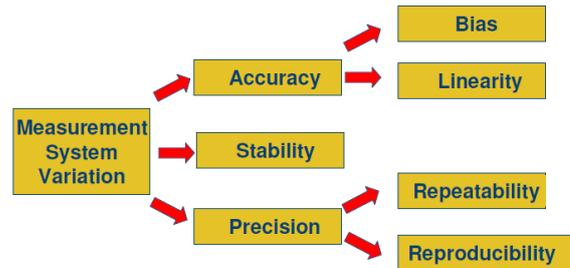
Fig. 3 Components of measurement variation [4].
