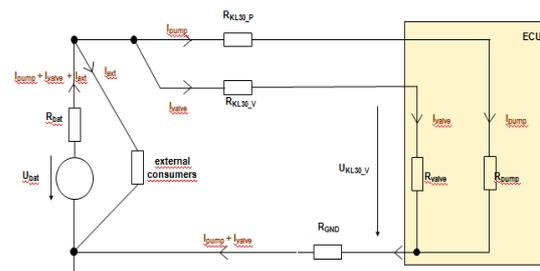
Figure 12. Simplified electrical circuit of vehicle for supplying braking system with voltage
