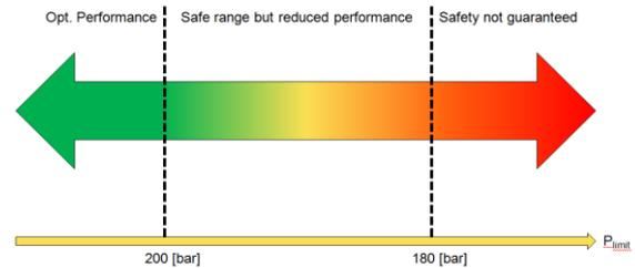
**Figure 18.** Defined thresholds for performance evaluation
