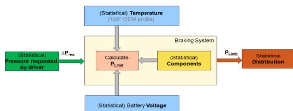
Figure 16. Structural overview of the Mote Carlo evaluation
