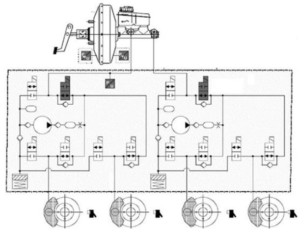
Figure 1. Braking system hydraulic layout
