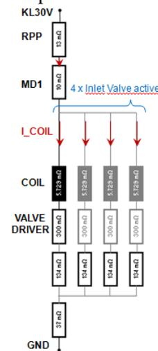
Figure 3. System electrical components schematic represented as resistances
