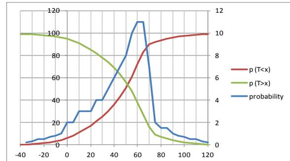
Figure 11. Shape of temperature distribution during vehicle lifetime
