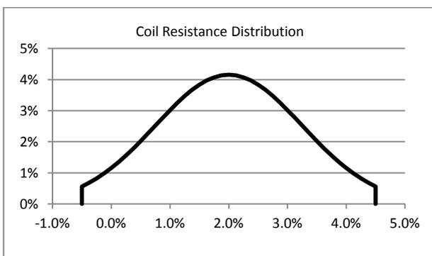
**Figure 6.** Shape of the distribution for valve coil resistance
