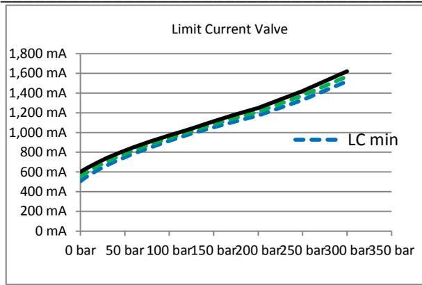
Figure 9. Limit current characteristic
