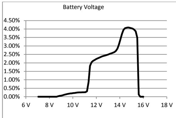
**Figure 13.** Probability distribution for vehicle battery voltage
