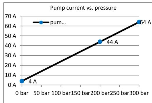
**Figure 15.** Pump current characteristic vs. pressure
