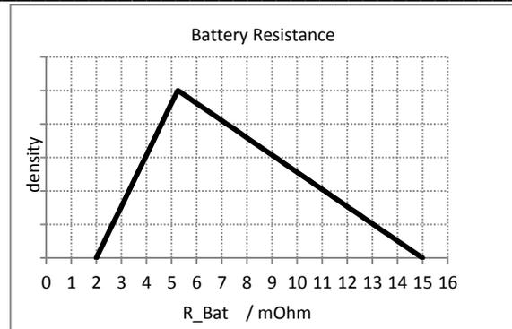
**Figure 14.** Probability distribution for vehicle battery internal resistance
