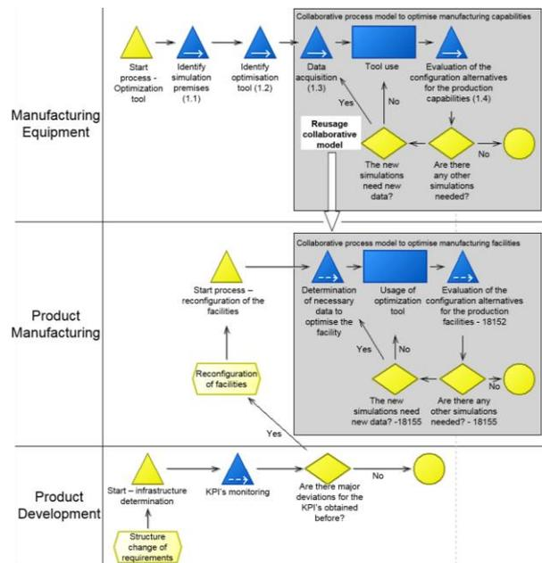
Fig. 7. The interaction of collaborative processes from the production added value chain with those from the production facilities value chain
