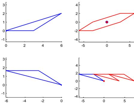
Fig.14. Optimal position of a triangle on the material strip.
