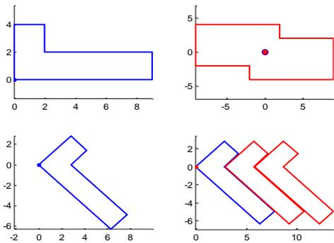
Figure 13. Optimal position of the “L” profile on the material strip.
