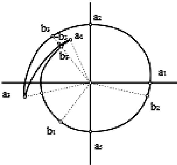
Figure 5. Ghosh diagram for A and B polygons.
