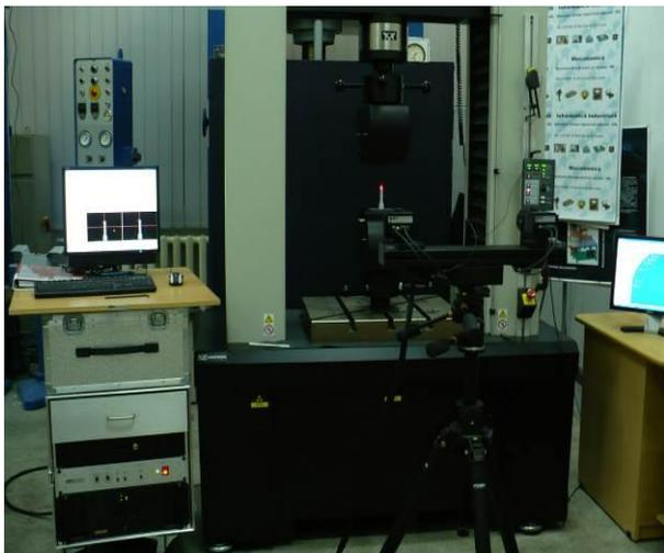
**Figure 1.** The experimental layout used for tensile test
