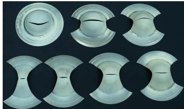
Figure 7 Test samples for forming limit curves
