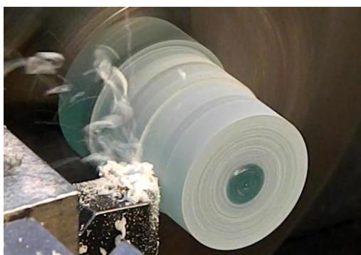
Figure 8. The chip fragmentation in the second cutting regime
