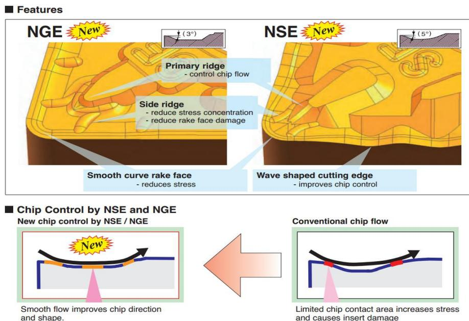
Figure 4. Special geometries and special control of chip evacuation
