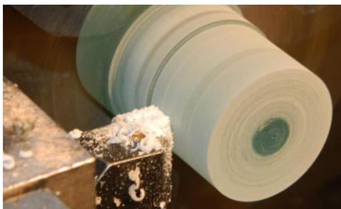
Figure 7. Material deposition in the first cutting regime
