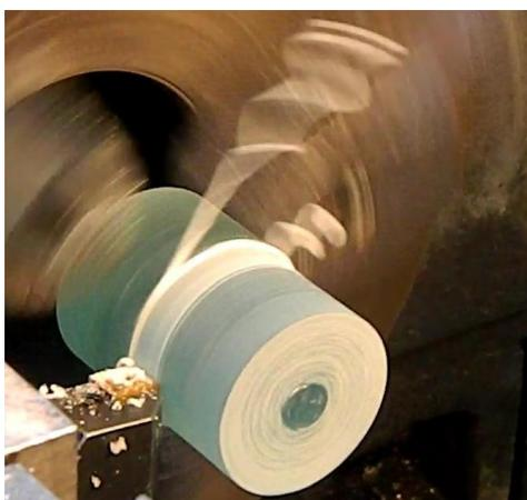
Figure 6. The chip fragmentation in the first cutting regime
