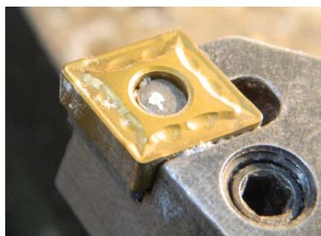
Figure 12. The material deposition after the last cutting regime
