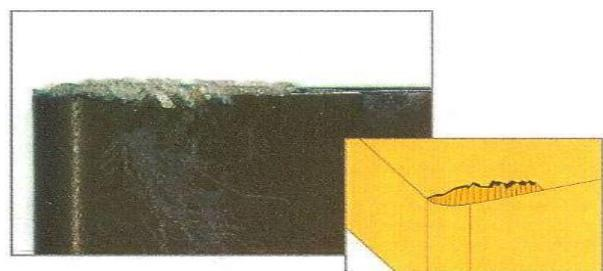
Figure 2. Wear due to deposits on the edge
