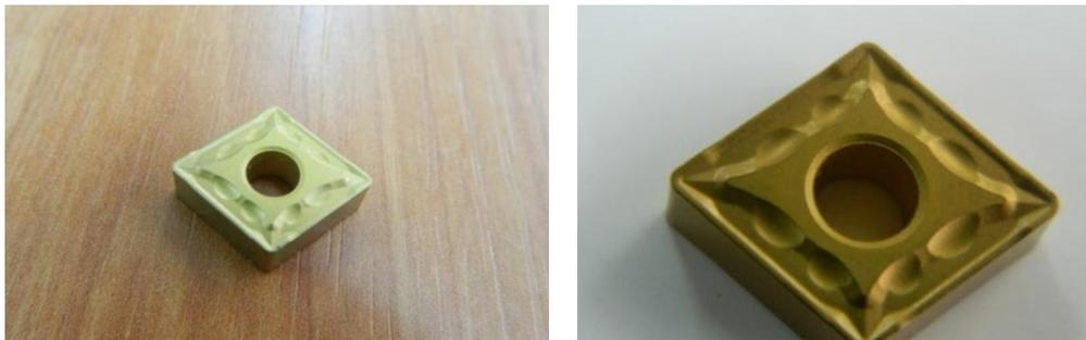
Figure 3. The SUMITOMO inserts (cutting tool)
