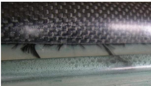
Figure 3. The excess of the resin after polymerization
