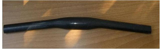
**Figure 4.** The carbon fibre/epoxy handlebar
