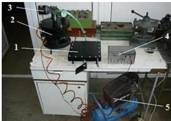
Figure 2. Experimental installation of RTM
