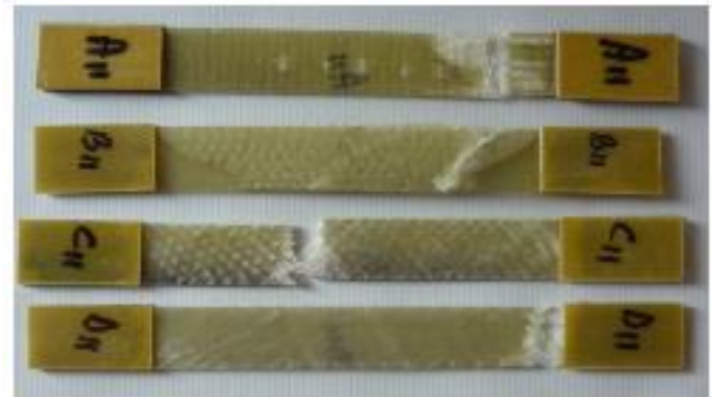
Figure 6. Specimens subjected to tensile strength
