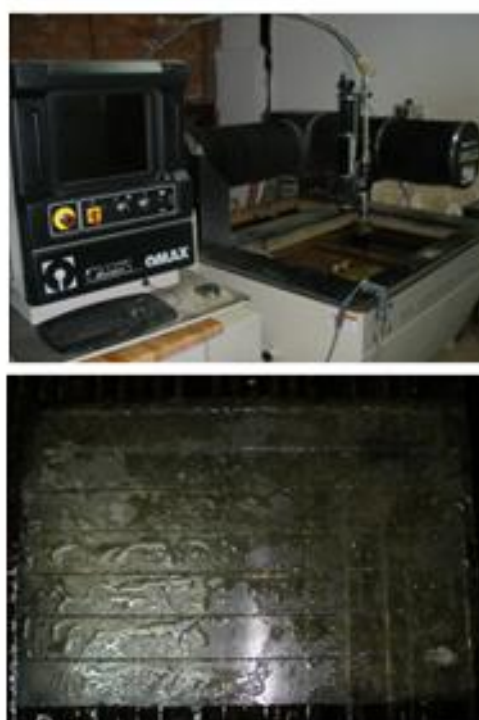
Figure 3. Waterjet Cutting Machine OMAX Jet Machining Center 2626
