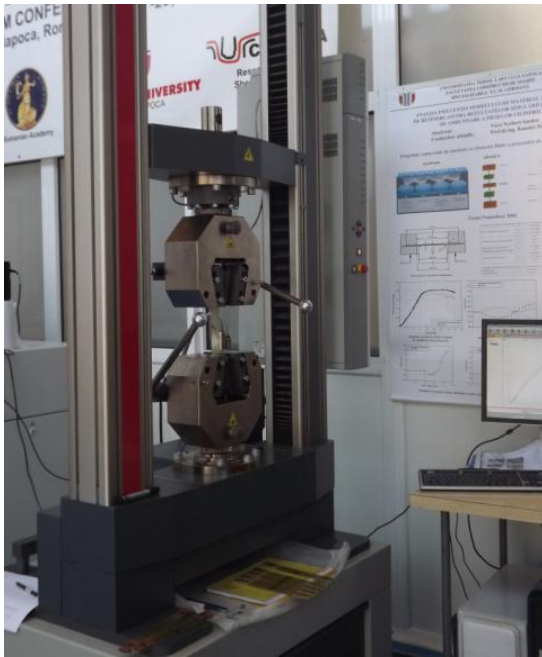
Figure 5. Tensile test machine Zwick/Roell Z150
