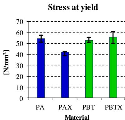
Figure 8. Values characterizing the stress at yield of the tested materials
