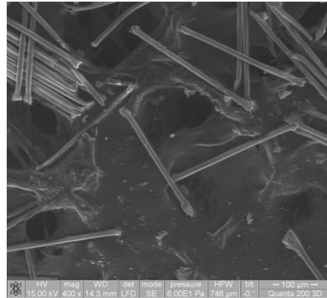
Figure 5. Aramid fibers before being added into the polymer (background: adhesive carbon tape G3939A)
