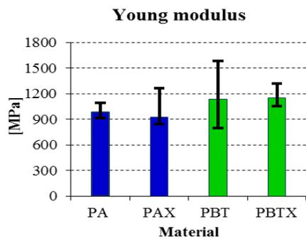
Figure 4. Young modulus for the tested materials ( $v=20$  mm/min)
