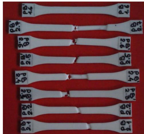
b) Samples made of PBT
