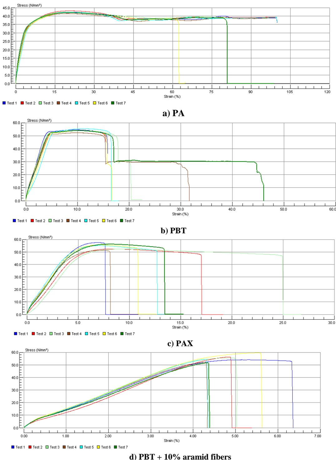
Figure 3. Dependence of strain on applied load (v=20 mm/min)
