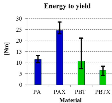
Figure 7. Energy at yield (a) and energy at break (b) for the tested materials
