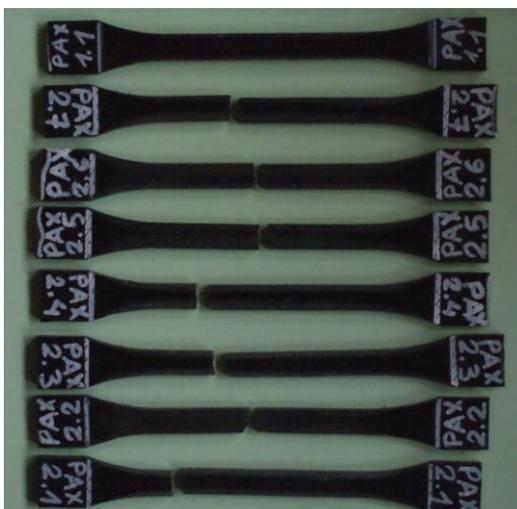
c) Samples made of PA + 10% aramid fibers
