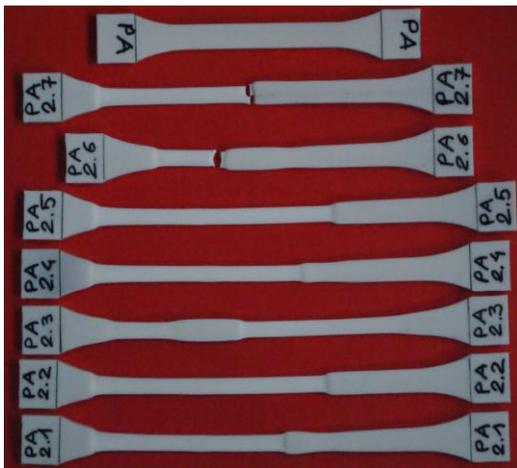
a) Samples made of PA were tested till 100% strain
