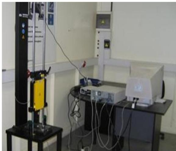
Figure 2. The Dynatup Model 8200 Impact Test
