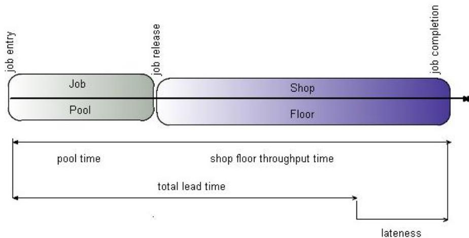
Figure 2. Lead time components with controlled release
