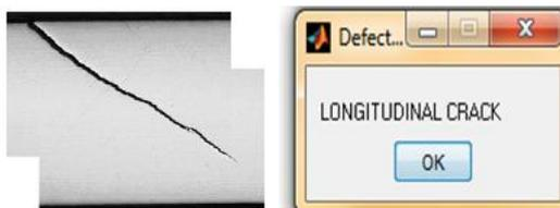
Figure 16. Longitudinal crack defect in the input image.
