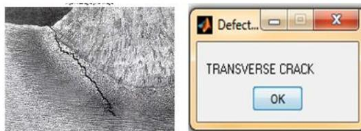
Figure 17. Transverse defect in the input image
