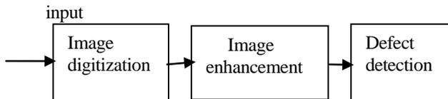
**Figure 2. Block diagram of the automatic interpretation system**
