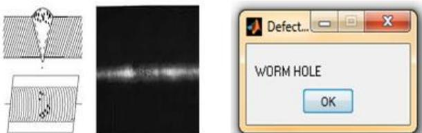
Figure 15. Worm hole defect in the input image.
