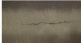
**Figure 1. Radiography image with weld defects**
