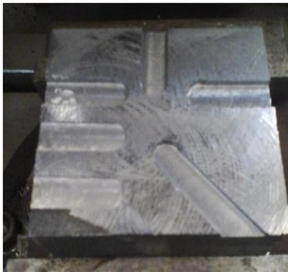
**Fig. 3. The blank after milling process**
