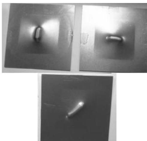
Fig. 6. The parts obtained through incremental forming
