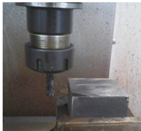
Fig. 2. The blank and the tool on CNC milling machine
