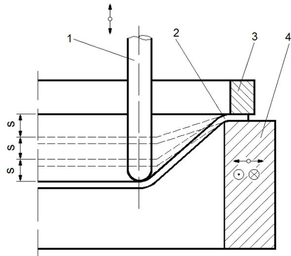
Fig. 1. Process principle of incremental forming
