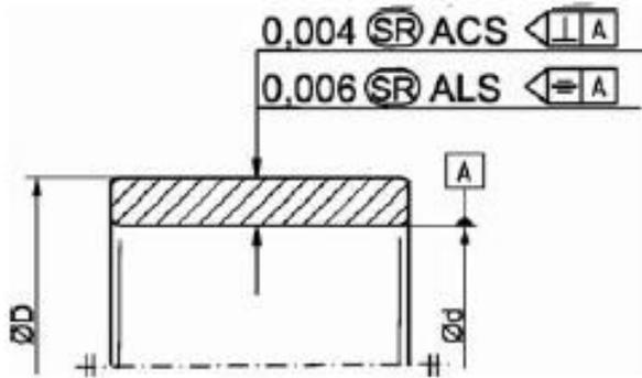
Fig. 3. Example of the use of a specification modifier for cylindrical surface
