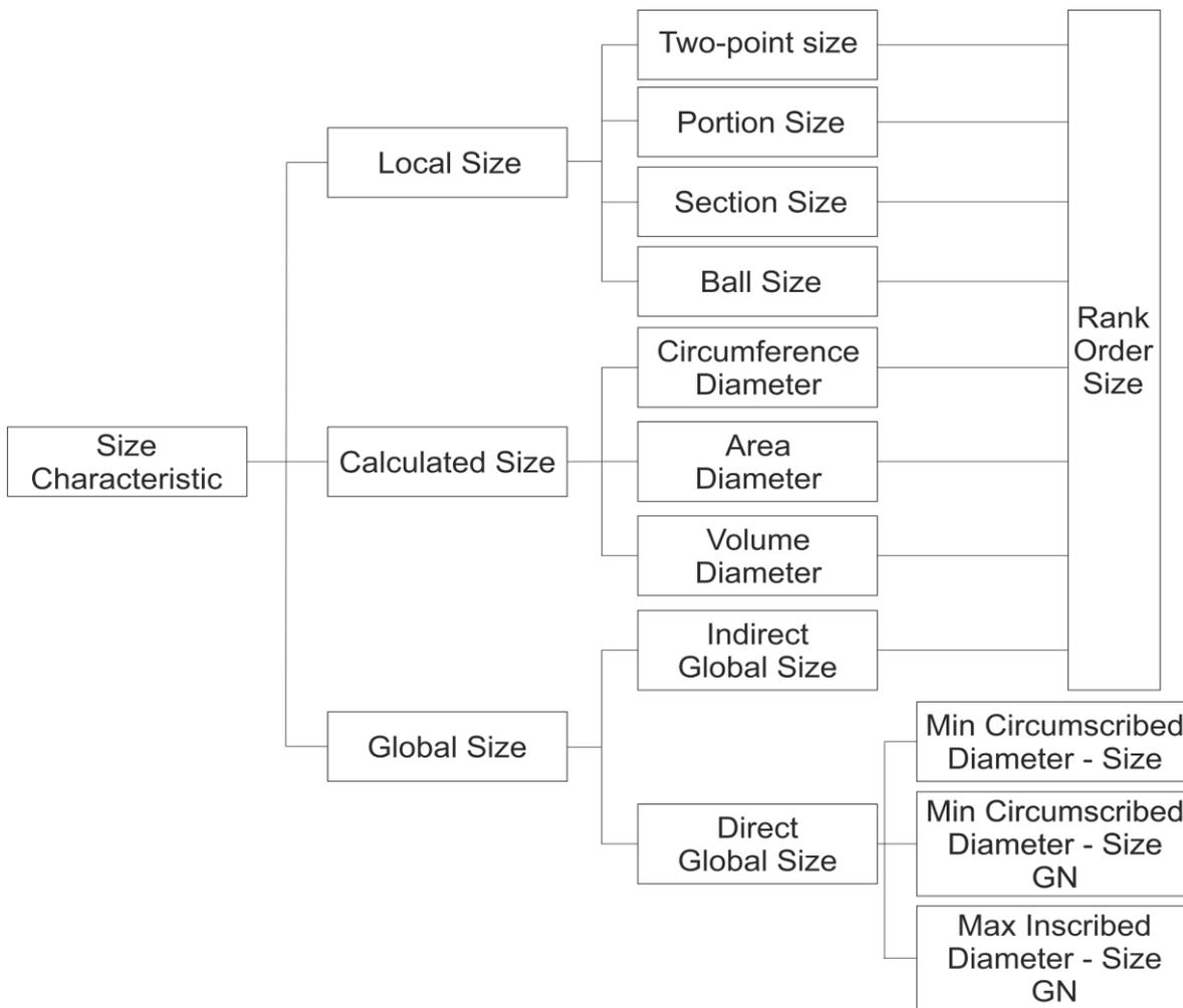
Figure 1. Overview diagram for size (ISO/DIS 14405-1, 2011)
