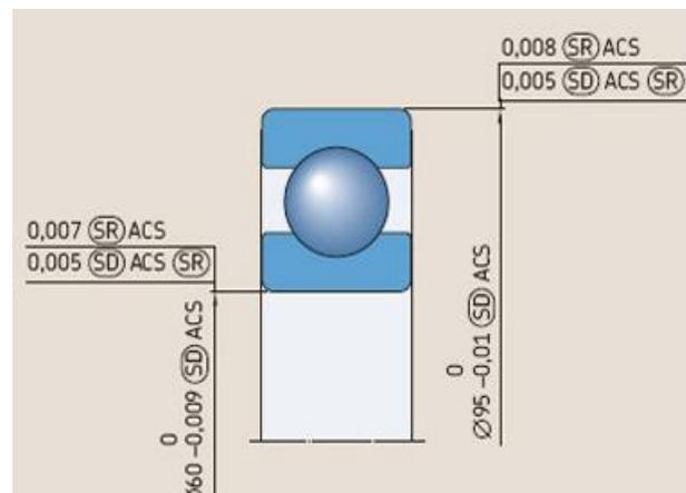
Figure 2. Example of the use of a specification modifier for bearings
