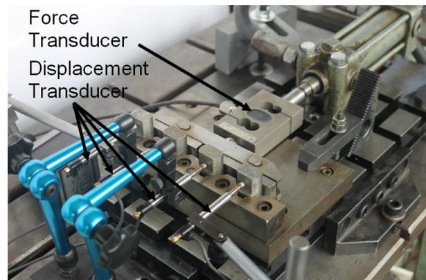
Figure 3. Parallel clamping fixtures
