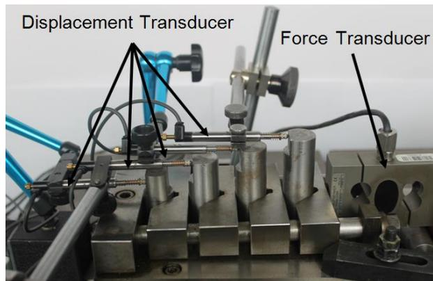
Figure 2. Serial clamping fixtures
