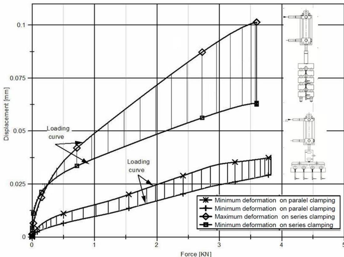
**Figure 6. The irregularity degree of the clamped workpieces serial and parallel clamping fixtures**
