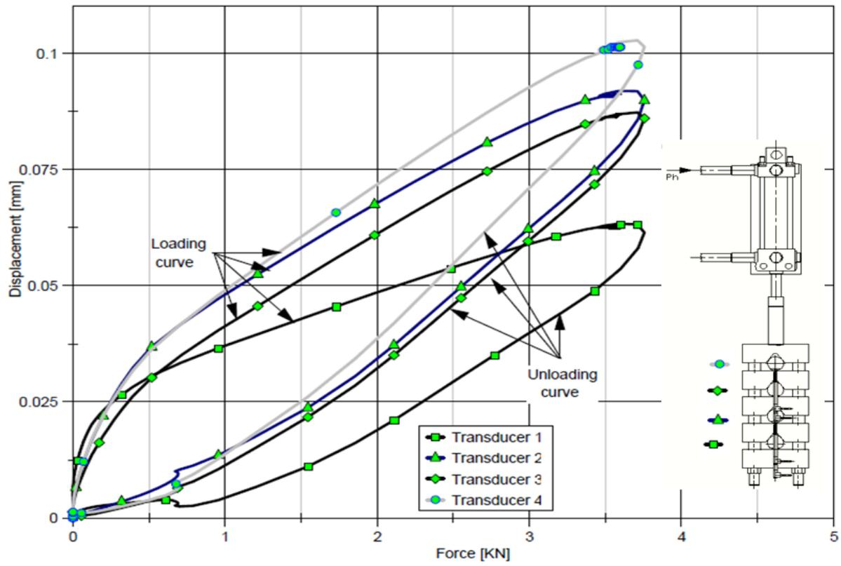
Figure 4. Displacements of workpieces clamped in serial clamping fixtures
