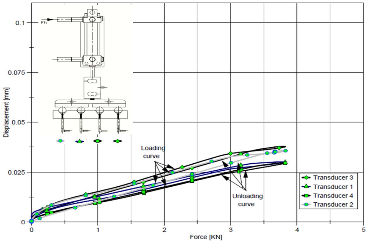
Figure 5. Displacements of workpieces clamped in parallel fixtures
