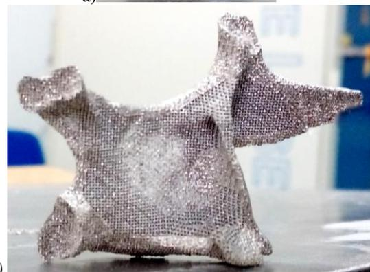
**Figure 7.** Future perspective: a) Medical grafts with variable porosity (2 types of lattice structures), b) Macro-porous implant with solid outer boundary SLM-manufactured
