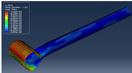
Figure 6. Strain energy distribution of the slit tube
