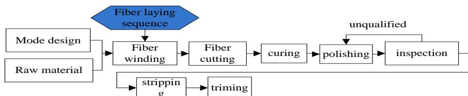
**Figure 1. Preparation of carbon Fibre thin-walled slit Tube**
