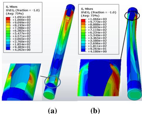
Figure 5. Buckling of slit tube (a) in the Z direction (b) in the Y direction
