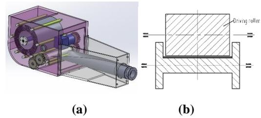
Figure 7. Design of the deployable boom (a) Driving mechanism (b) Driving roller
