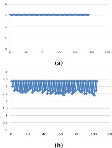
Figure 8. Velocity fluctuation (a) Preload is 50N and axial load is 15N (b) Preload is 50N and axial load is 45N
