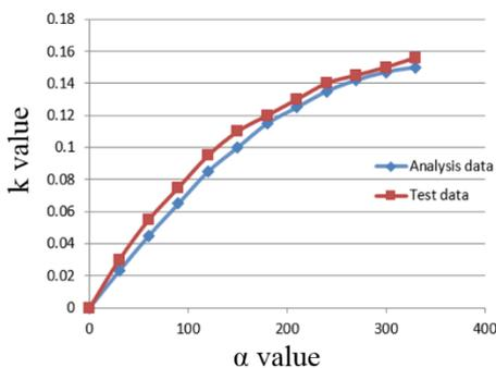
Figure 4. Relationship between the opening angle  $\alpha$  and k
