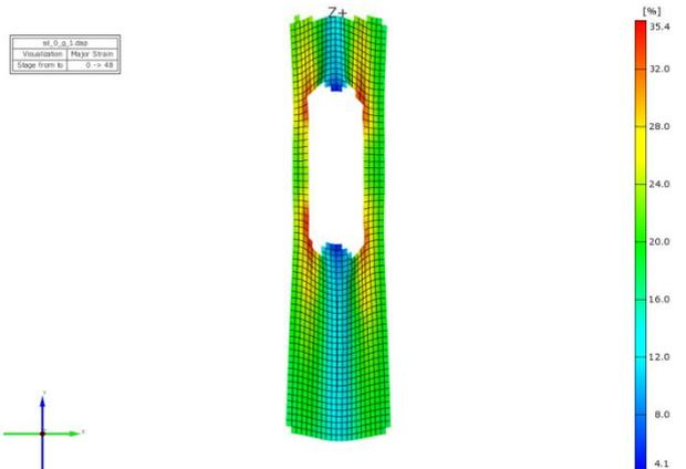
Figure 13 The values of major strain for a specimen with stress concentrator loaded on the warp direction
