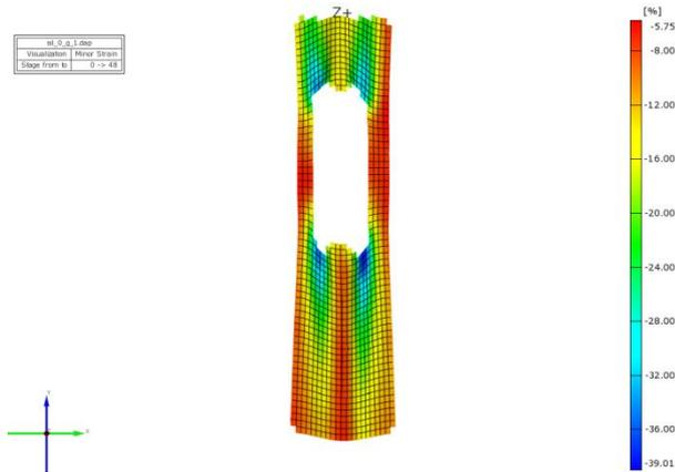
Figure 14 The values of minor strain for a specimen with stress concentrator loaded on the warp direction
