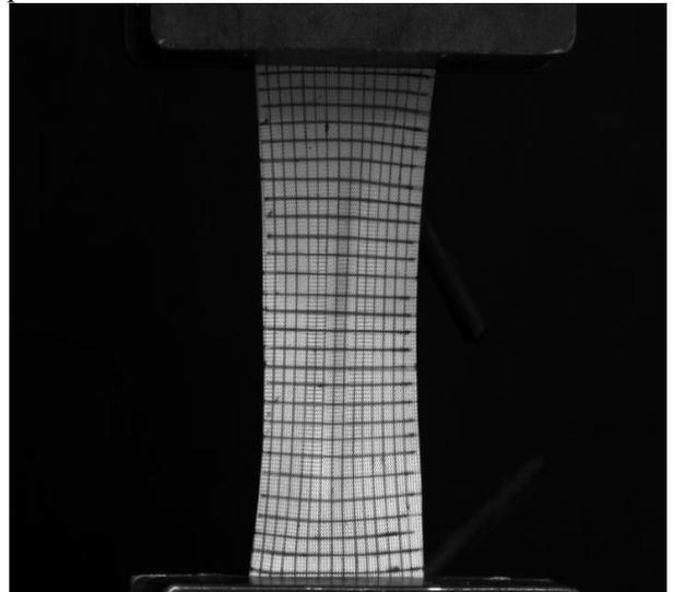
**Figure 1. Specimen prepared for experiments with a linear grid deposited on the analyzed surface**
