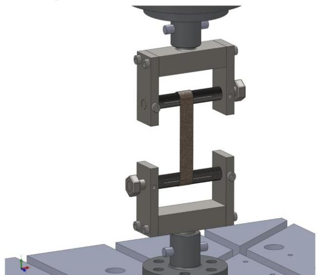
**Figure 2. Experimental layout for uniaxial tension tests**
