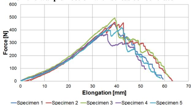
**Figure 8 Force-elongation curve for specimens loaded on the weft direction with stress concentrator**
