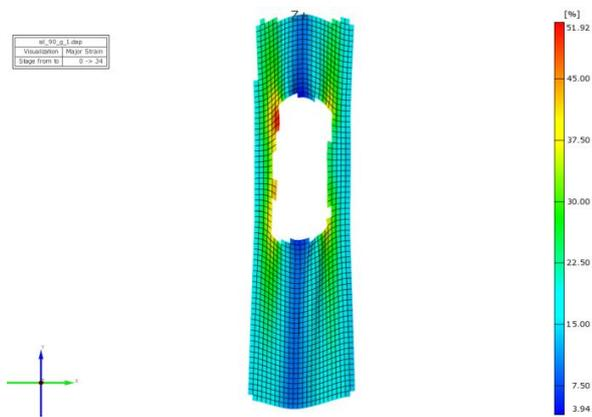
Figure 15 The values of major strain for a specimen with stress concentrator loaded on the weft direction
