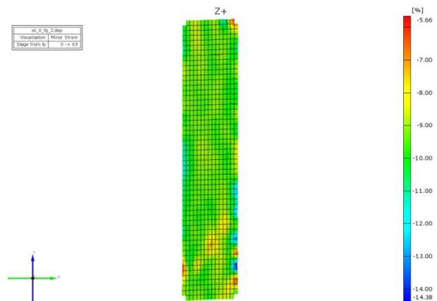
Figure 12 The values of major strain for a specimen without stress concentrator loaded on the weft direction
