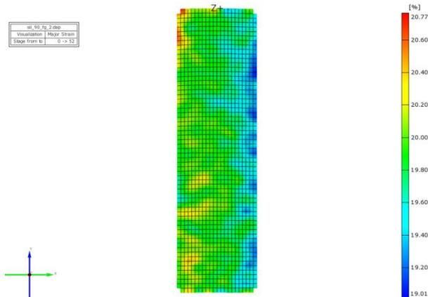
Figure 9 The values of major strain for a specimen without stress concentrator loaded on the warp direction
