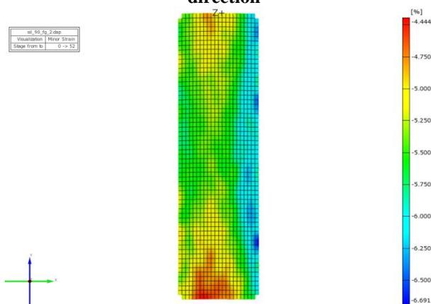
Figure 10 The values of minor strain for a specimen without stress concentrator loaded on the warp direction
