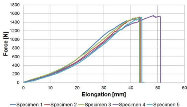
**Figure 5 Force-elongation curve for specimens loaded on the warp direction without stress concentrator**
