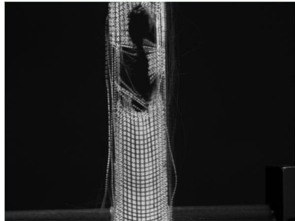
Figure 3. Fracture type for a PA 6.6 silicone coated fabric specimen loaded on the warp direction
