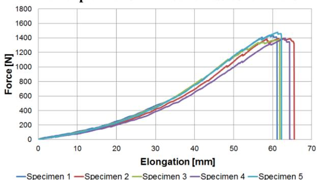
**Figure 6 Force-elongation curve for specimens loaded on the weft direction without stress concentrator**
