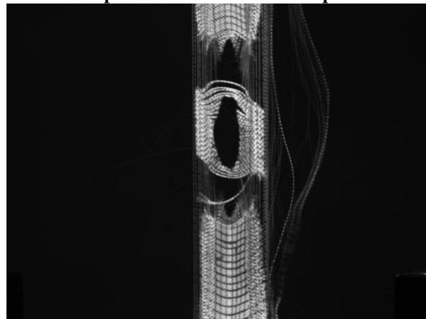
Figure 4. Fracture type for a PA 6.6 silicone coated fabric specimen loaded on the weft direction
