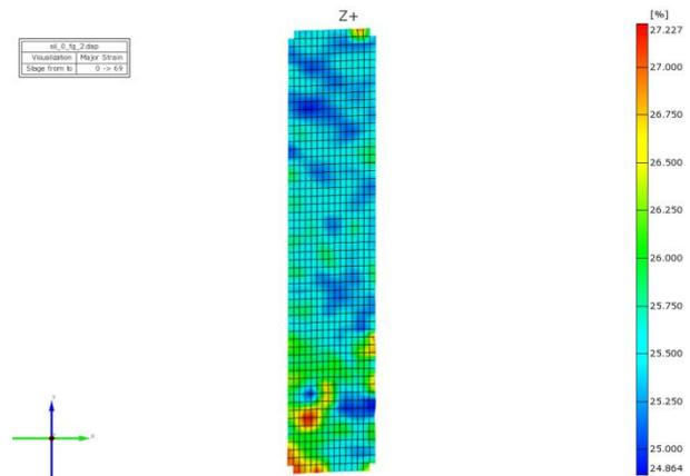
Figure 11 The values of major strain for a specimen without stress concentrator loaded on the weft direction
