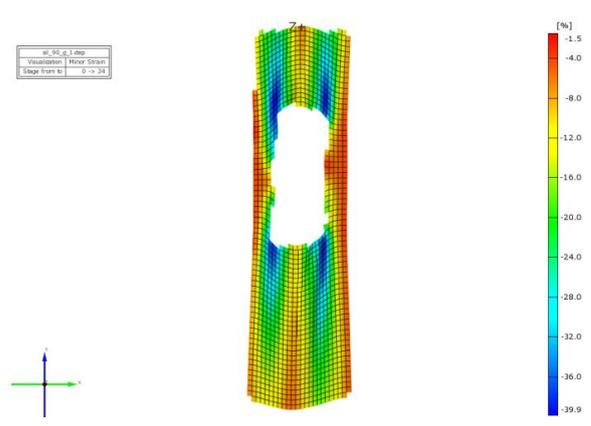
Figure 16 The values of minor strain for a specimen with stress concentrator loaded on the weft direction
