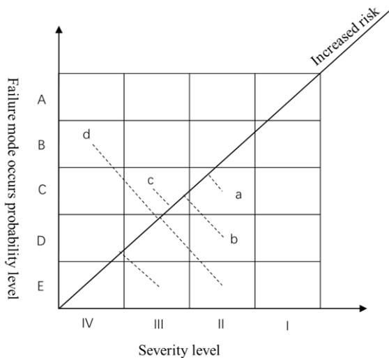
**Fig. 3** Logging hydraulic drive system hazard matrix diagram
