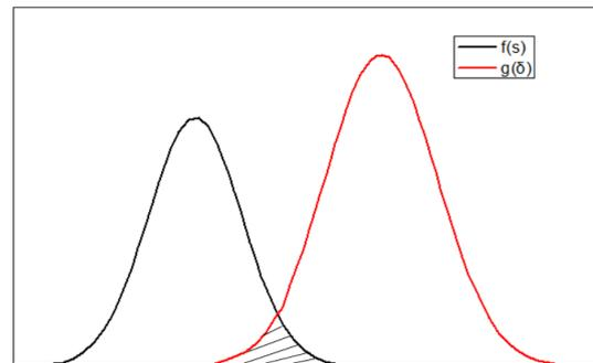
Fig.5 Stress-strength interference model
