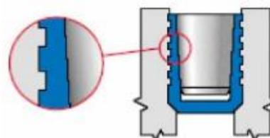
**Fig. 4** Body expansion seal
