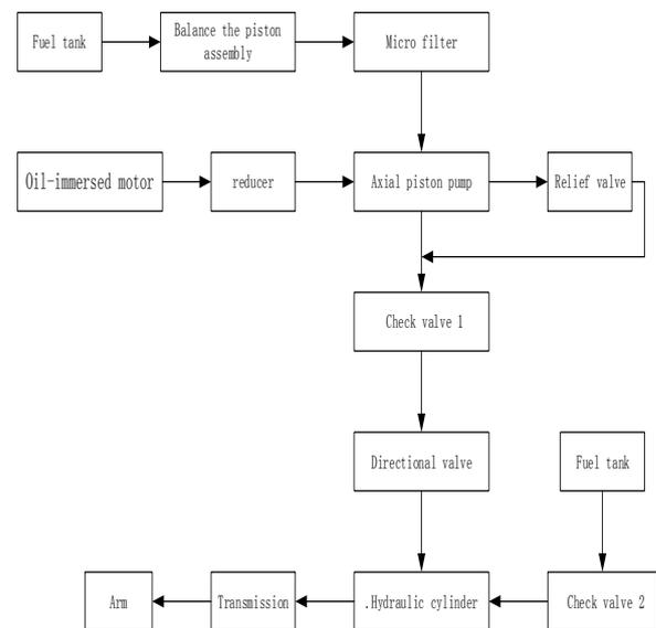
Fig. 2 System function and structure diagram
