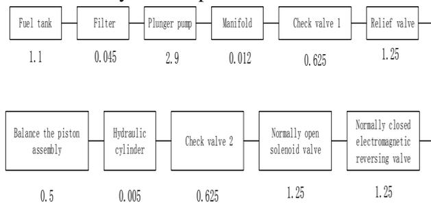
Fig 1 Toolbox hydraulic drive system reliability diagram
