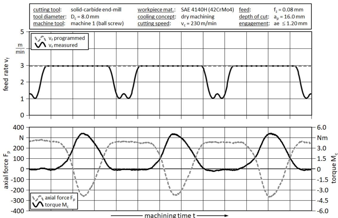
Figure 2. Experimental results for static milling of SAE 4140H with ball screw drives
