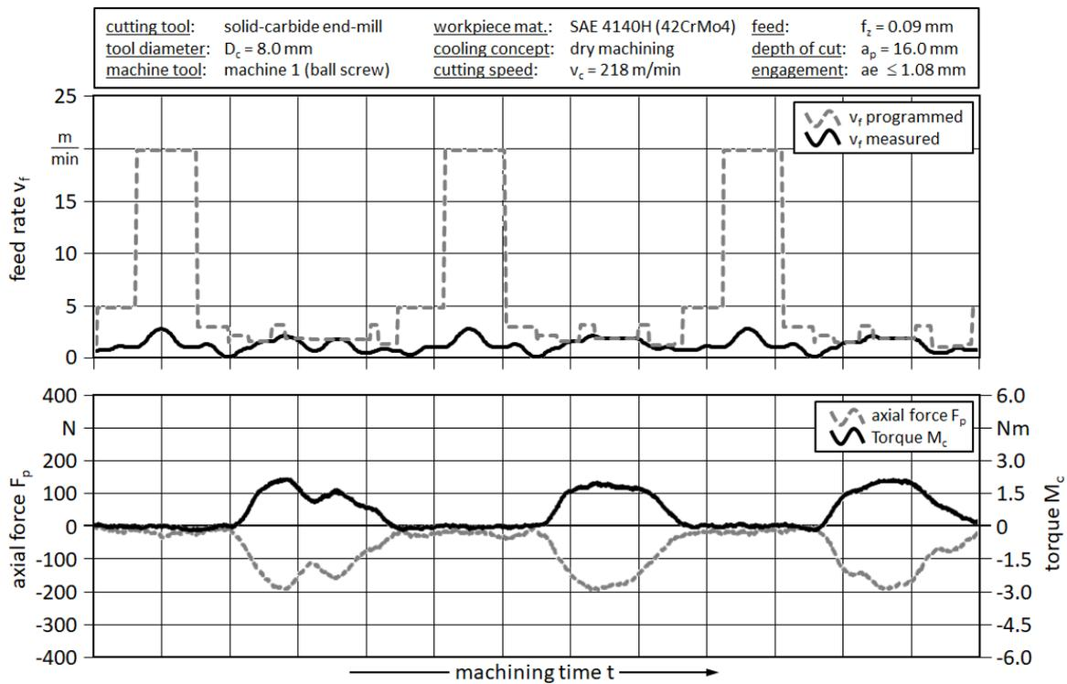
Figure 3. Experimental results for dynamic milling of SAE 4140H with ball screw drives
