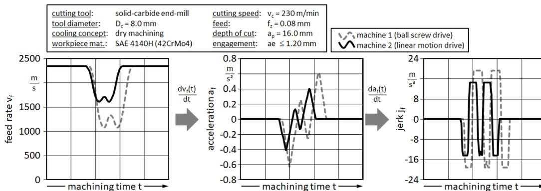
Figure 4. Feed rate, acceleration and jerk for static milling on different machine tools
