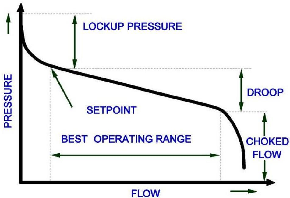
Figure 8: Direct Acting Pressure Regulator Operating Map
