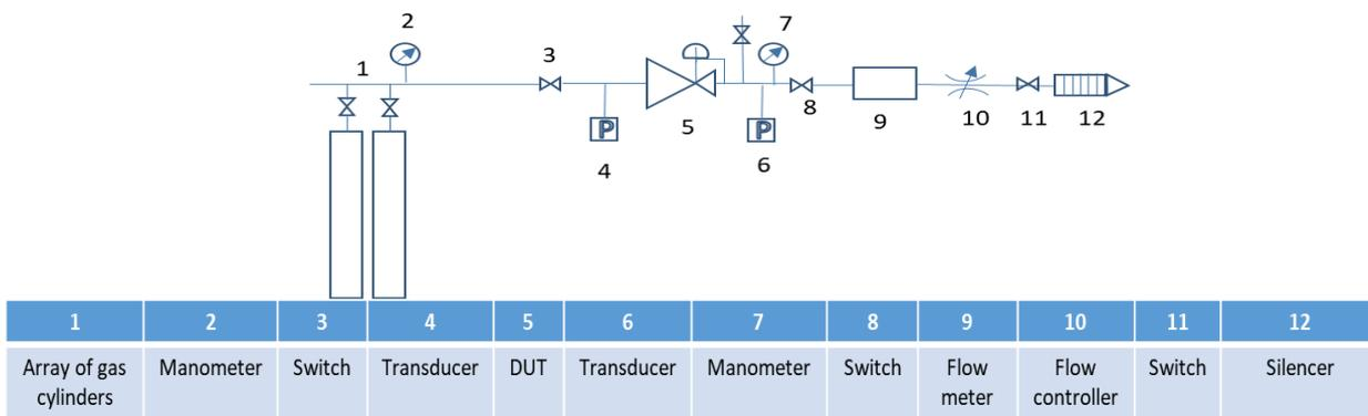
Figure 6. Test set-up 2
