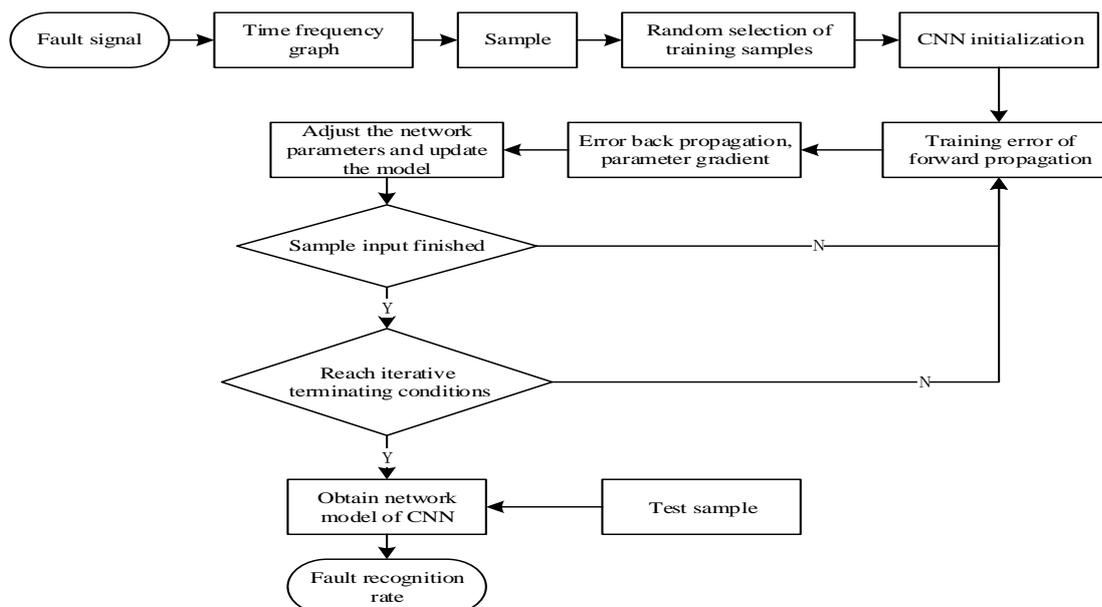
Figure 1. Process of fault diagnosis for gearbox
