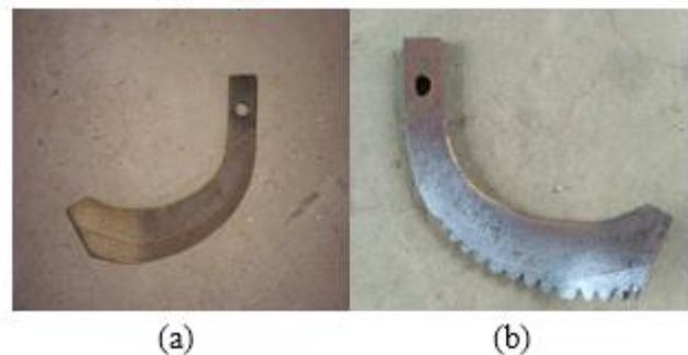
**Figure 3. Pictures of the prototype and bionic rotary blades** (a. Picture of the rotary cutting tool; b. Picture of the prototype rotary cutting tool)
