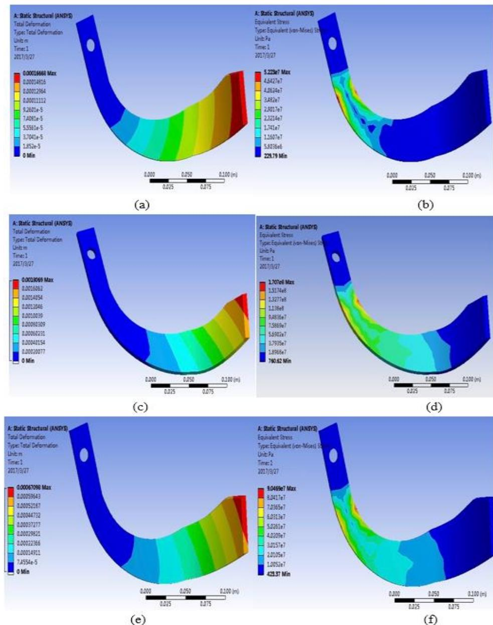
**Figure 4. Force analysis diagrams of the prototype rotary blade** (a. Total deformation of the loaded prototype rotary blade side edge; b. Total stress of the loaded prototype rotary blade side edge; c. Total deformation of the loaded prototype rotary blade sidelong edge; d. Total stress of the loaded prototype rotary blade sidelong edge; e. Total deformation of the loaded prototype rotary blade full edge; f. Total stress of the loaded prototype rotary blade full edge)
