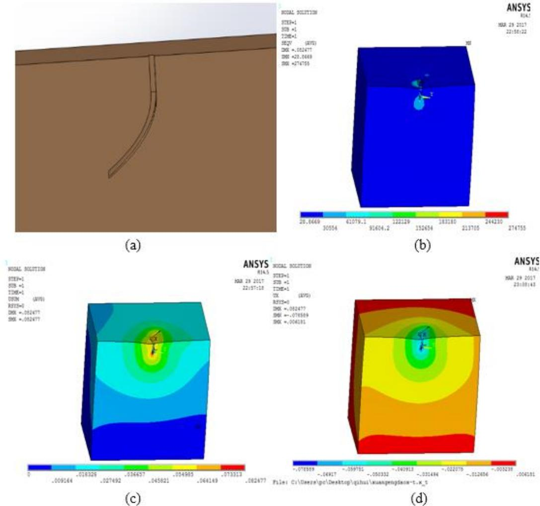
**Figure 6. Soil statics analysis diagrams of the prototype rotary blade** (a. Soil model for the prototype rotary blade with the maximum tillage depth; b. Diagram of total soil stress for the prototype tool used in rotary tillage; c. Diagram of total soil deformation for the prototype tool used in rotary tillage; d. Diagram of soil deformation in the forward direction for the prototype tool used in rotary tillage)
