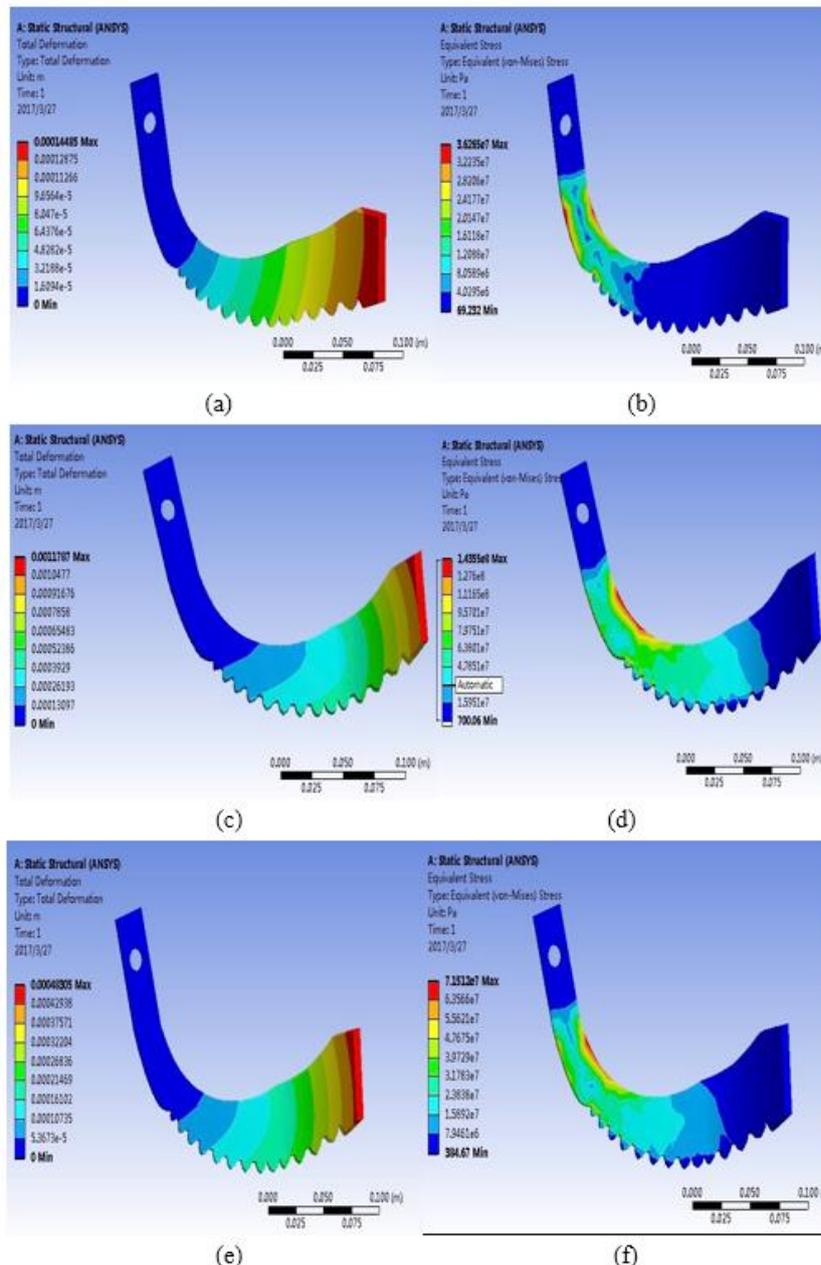
**Figure 5.** Force analysis diagrams of the bionic rotary blade (a. Total deformation of the loaded bionic rotary blade side edge; b. Total stress of the loaded bionic rotary blade side edge; c. Total deformation of the loaded bionic rotary blade sidelong edge; d. Total stress of the loaded bionic rotary blade sidelong edge; e. Total deformation of the loaded bionic rotary blade full edge; f. Total stress of the loaded bionic rotary blade full edge)
