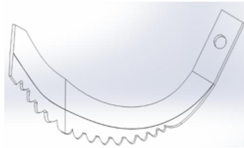
**Figure 2. Schematic diagram of the bionic rotary cutting tool**
