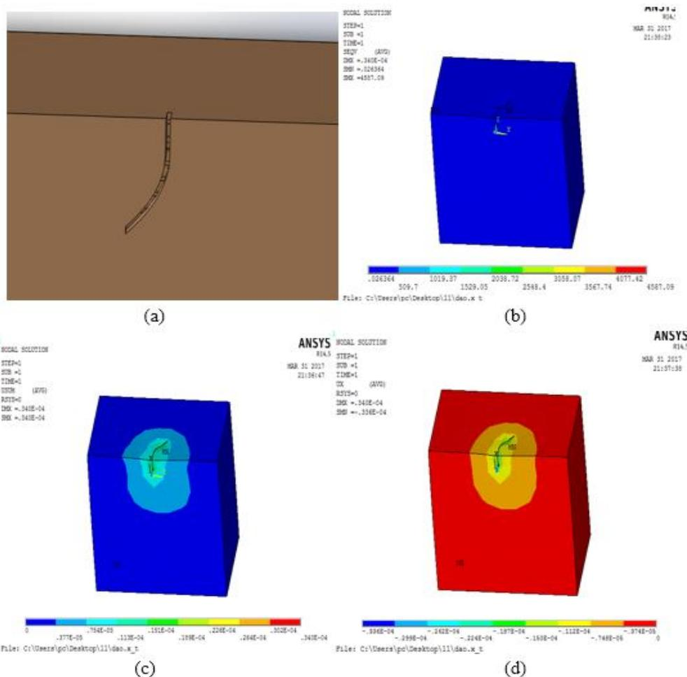
**Figure 7. Soil statics analysis diagrams of the bionic rotary blade** (a. Soil model for the bionic rotary blade with the maximum tillage depth; b. Diagram of total soil stress for the bionic tool used in rotary tillage; c. Diagram of total soil deformation for the bionic tool used in rotary tillage; d. Diagram of soil deformation in the forward direction for the bionic tool used in rotary tillage)
