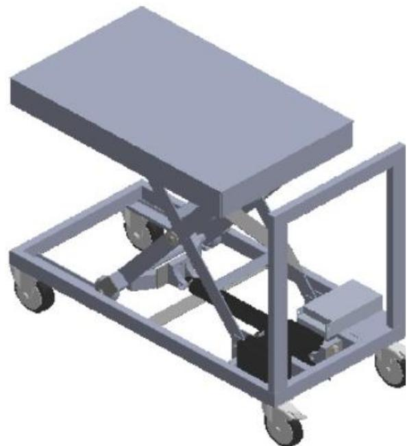
Figure 1. Schematic view of the subject scissor lift table/cart
