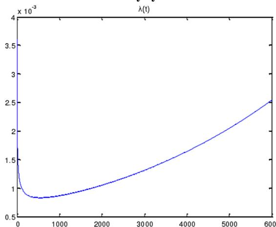
Figure 4. The failure rate function graph of the tool library system
