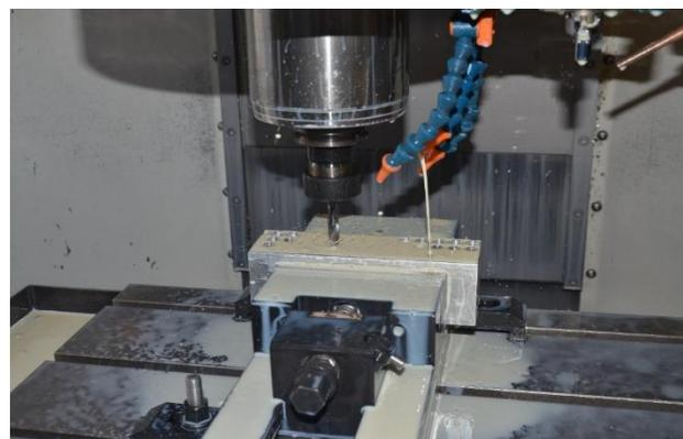
**Figure 1. Drilling operation of EN AW-2007 on HAAS VF 2**
