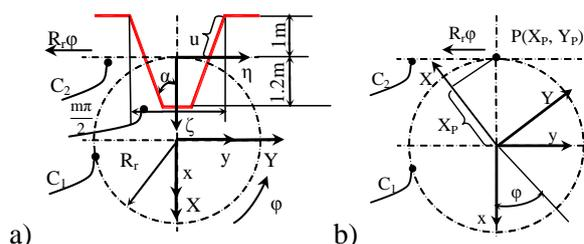
**Figure 1.a) The generation of rotor front view profile; b) Gearing pole coordinates, in XY system**
