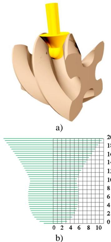
Figure 5. a) Relative position of cylindro-frontal tool axis to the XYZ system; b) Axial section of the tool
