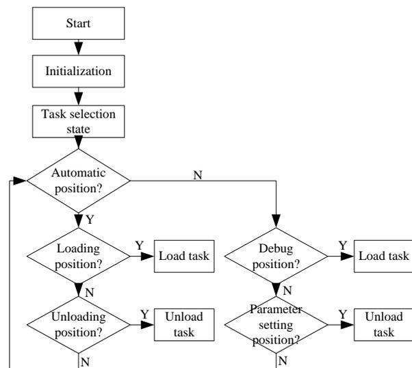
Figure 3. Flow chart of the automatic control programme
