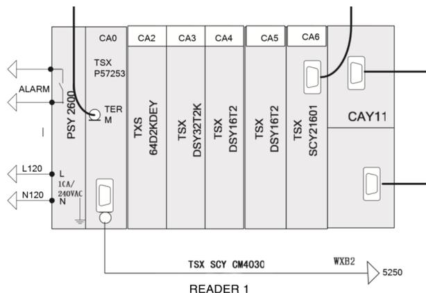
Figure 2. Controller composition diagram
