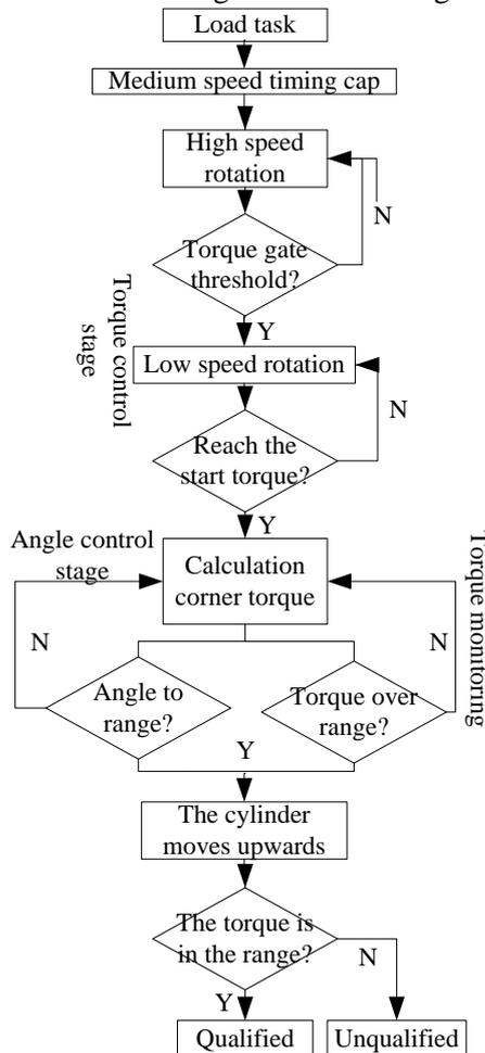
Figure 4. Flow chart of the loading task
