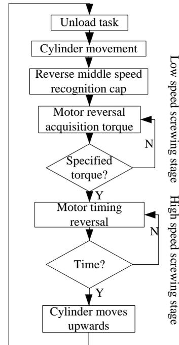
Figure 5. Flow chart of the unloading task
