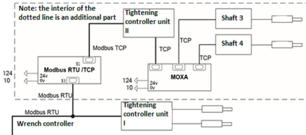
Figure 1. Tightening control structure diagram
